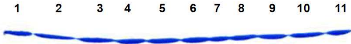
Figure 3- 5. SDS-PAGE analysis of BSA precipitation by TCA. Lane: 1, 2.00% w/v TCA; 2, 5.78% w/v TCA; 3, 1.35 %w/v; 4, 3.95%w/v TCA; 5, 4.35%w/v TCA; 6, 2.50% w/v TCA; 7, 0.95%w/v TCA; 8, 5.30%w/v TCA; 9, 3.18% TCA; 10, 10.00 %w/v TCA; 11, 20.00% w/v TCA.
