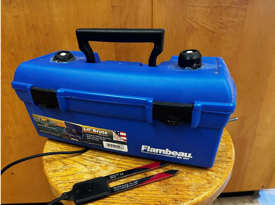
Image 2.2. Image of the box that was used to house and protect the data logger systems throughout the course of the study.
