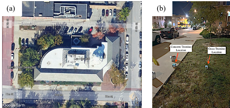
Figure 25: (a) An aerial photo of Lee's Hall BH-08 site location, and (b) is a photo of the Tromino set up before data acquisition.
