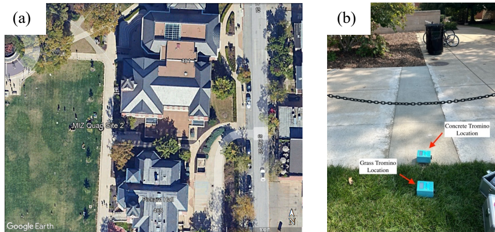
Figure 29: (a) An aerial photo of MIZ Quad Site 2 site location, and (b) is a photo of the Tromino set up before data acquisition.
