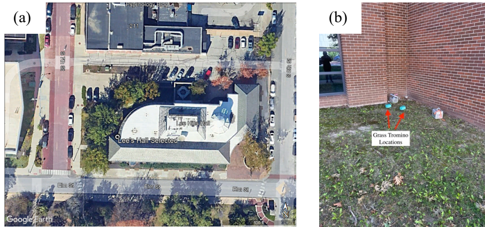
Figure 27: (a) An aerial photo of Lee's Hall Selected site location, and (b) is a photo of the Tromino set up before data acquisition.
