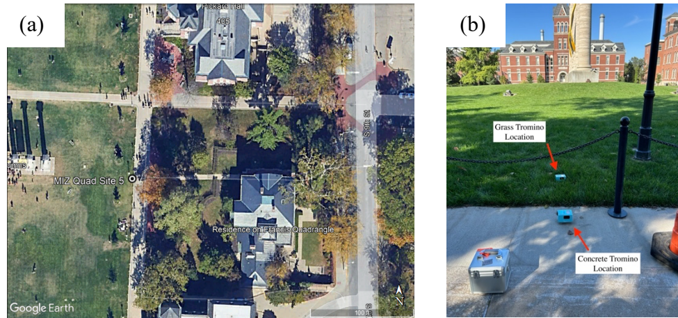
Figure 32: (a) An aerial photo of MIZ Quad Site 5 site location, and (b) is a photo of the Tromino set up before data acquisition.
