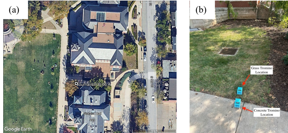
Figure 23: (a) An aerial photo of Journalism BH-06 A site location, and (b) is a photo of the Tromino set up before data acquisition.
