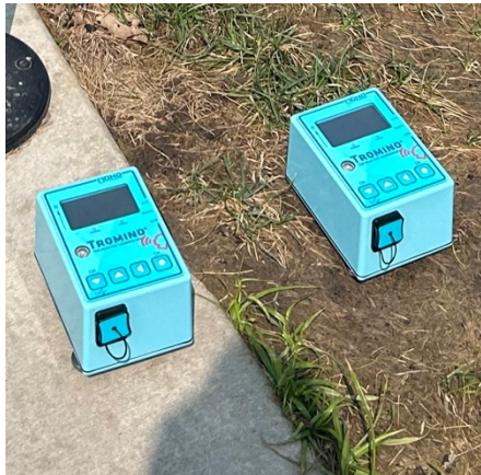
Figure 7: Tromino device used in data acquisition. Image of Tromino devices acquiring data on concrete and grass simultaneously at MIZ Quad Site 4.
