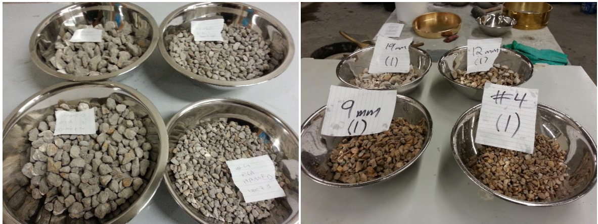
Figure 3.1 RCA Particles before Separating the Mortar (left) and after Separating the Residual Mortar (right)
