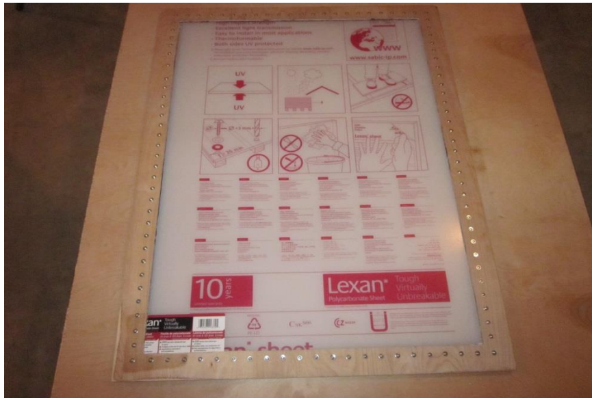
Figure 42 Inner Shell Window With Frame
