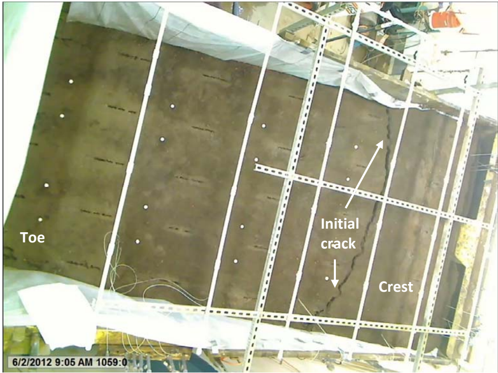
Figure 5.5 Second stage of unsaturated failure, SL2.
