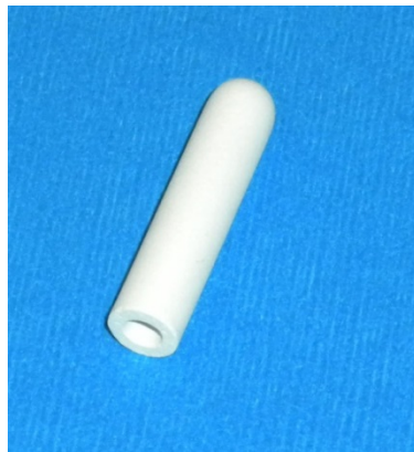
B-3 Porous ceramic tip of tensiometer.
