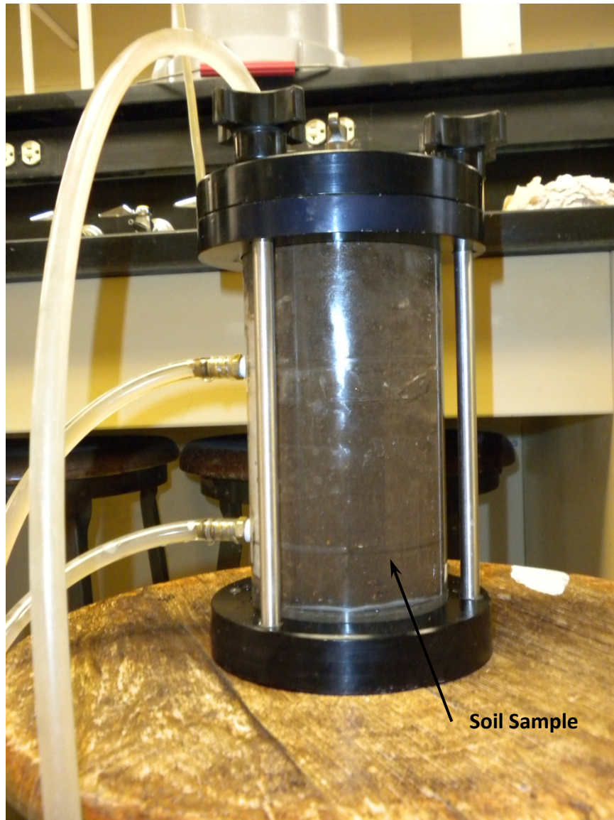
Figure 3.19 Sample of soil in permeameter.
