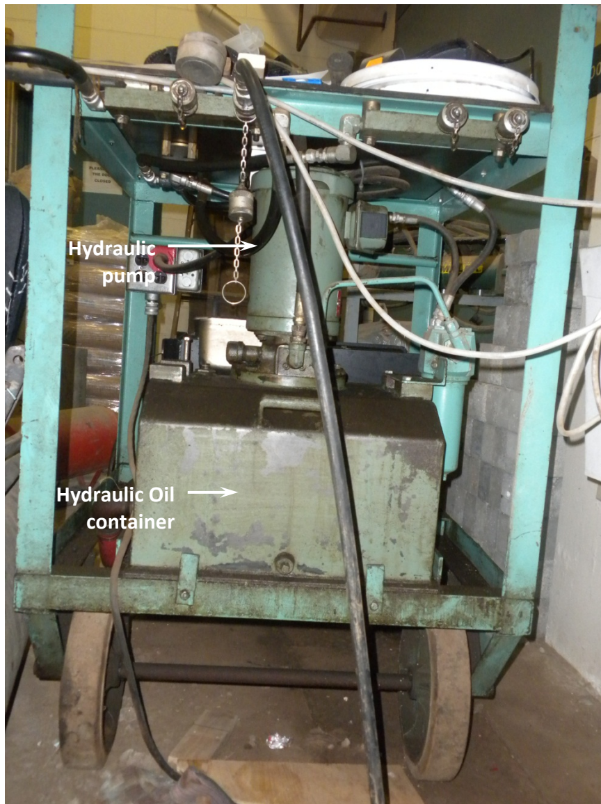
Figure 3.3 Hydraulic pump used to lift the model container.
