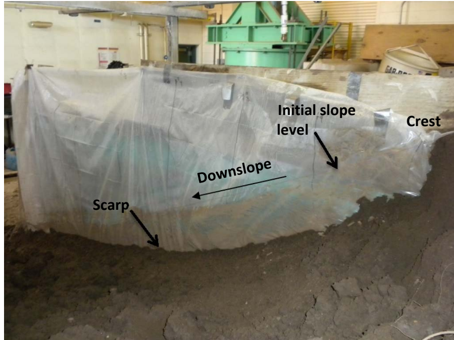
Figure 4.15 General view of failure shape SL2.
