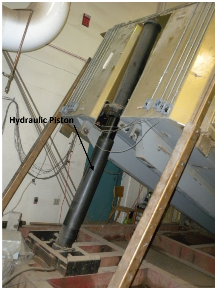
Figure 3.2 Hydraulic piston of the lifting mechanism.
