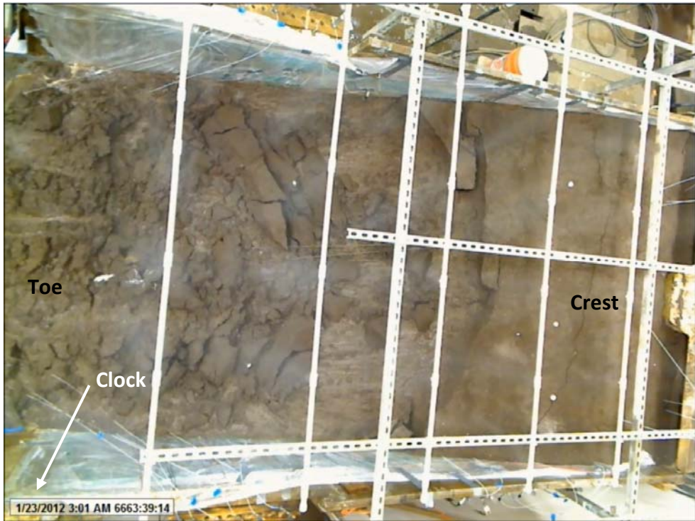
Figure 4.10 Top view of third stage of failure SL1.
