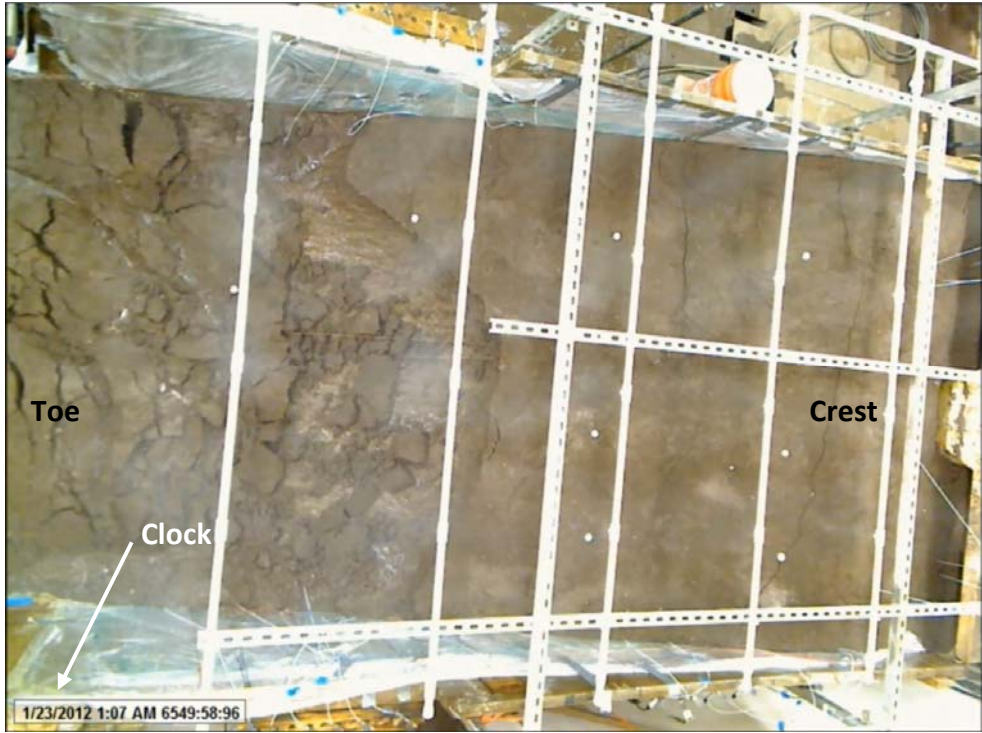
Figure 4.9 Top view of second stage of failure SL1.
