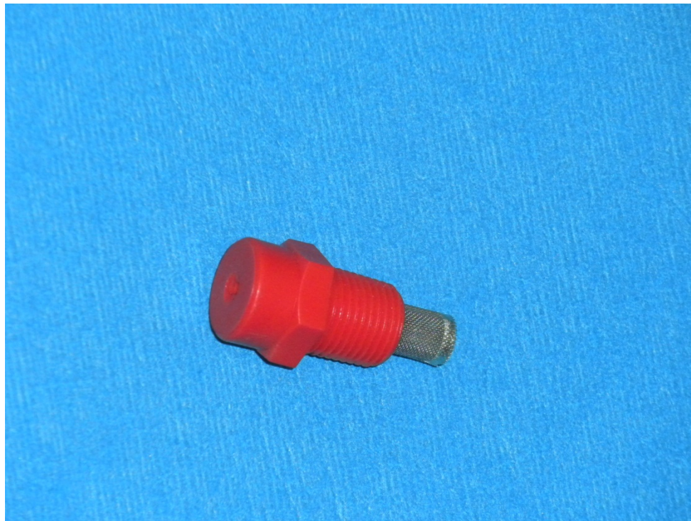
Figure 3.6 Picture of a nozzle used in precipitation system.
