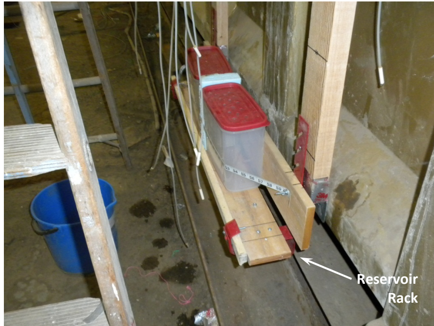
B-9 Water reservoirs to maintain the porous ceramic tips under water.
