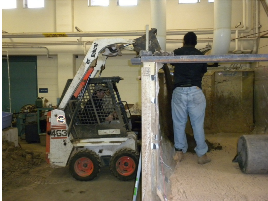
Figure 3.21 Placement of soil in model container.
