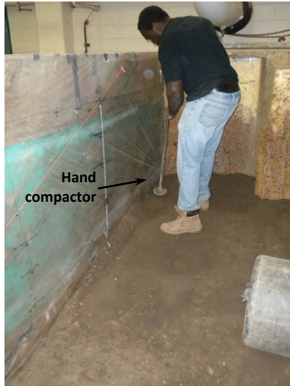
Figure 3.23 Hand compacting of soil along the edges of the container.
