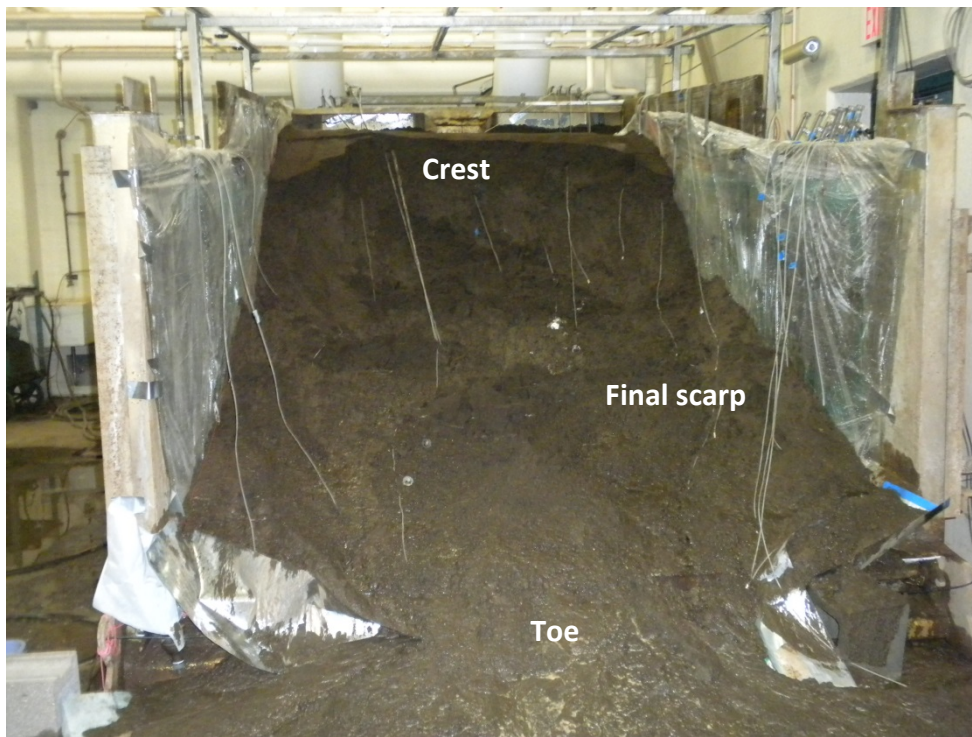
Figure 4.12 Front view of the last stage of failure SL1.
