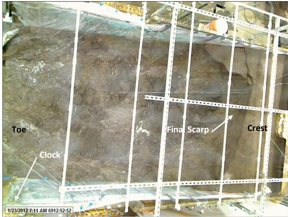
Figure 4.11 Top view of last stage of slope failure SL1.
