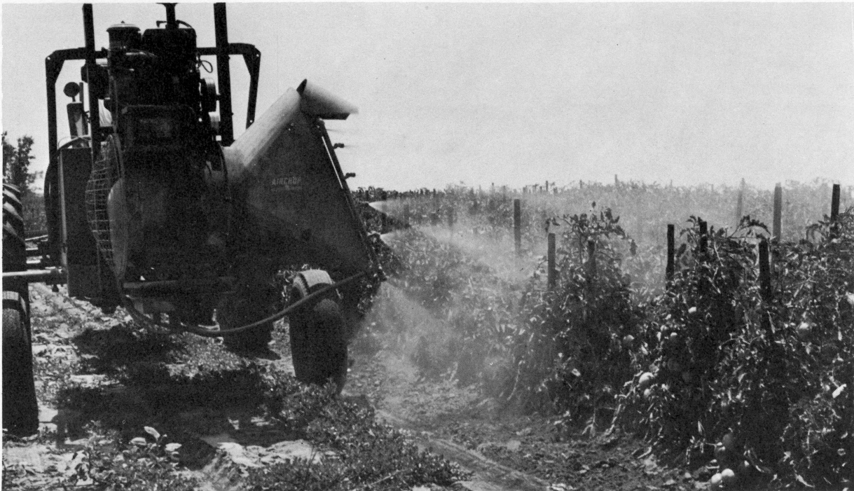
Air blast sprayer gives excellent control of insects and disease.
