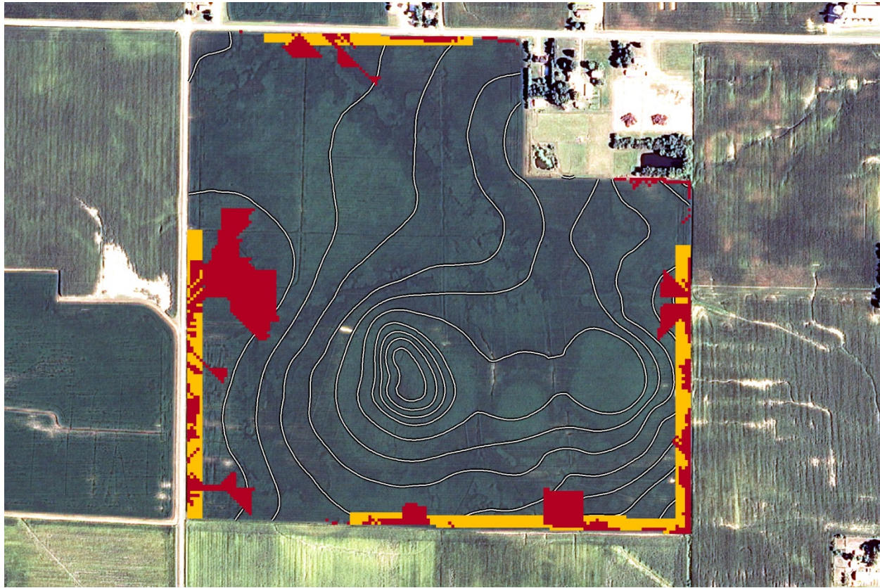
Figure 1. Aerial photo of a 59.3 ha field in Madison Co., IL showing 1-m contours and a constant-width (20-25 m) buffer (in yellow) having the same total area as the BufferBuilder design (in red). The sediment trapping efficiency of the constant-width configuration on a whole-field basis was estimated to be 35% while that of the BufferBuilder design was estimated to be 72%.
