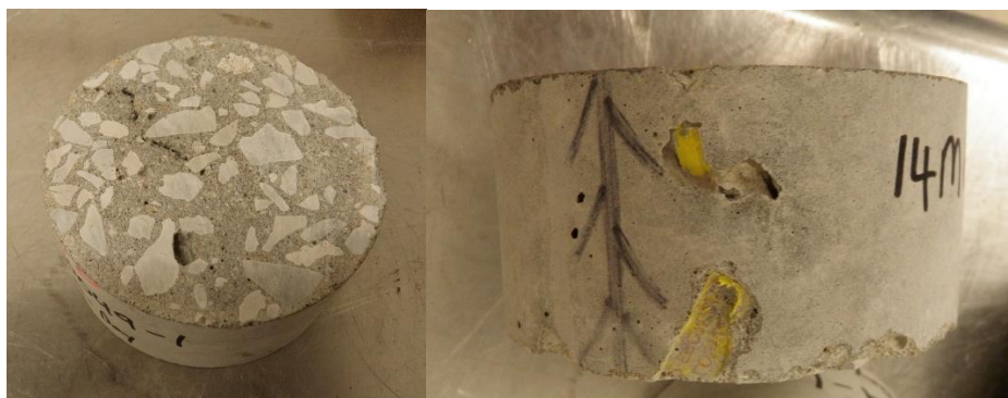
Figure 18. Field produced concrete cylinders with defects
