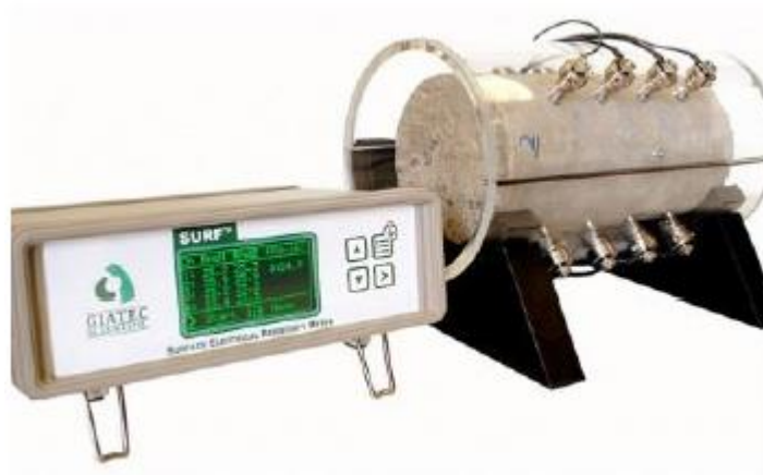
Figure 9. Giatec Surf surface resistivity meter (Giatec Scientific, 2015)
