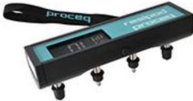
Figure 7. Proceq resipod surface resistivity meter (Proceq, 2015)
