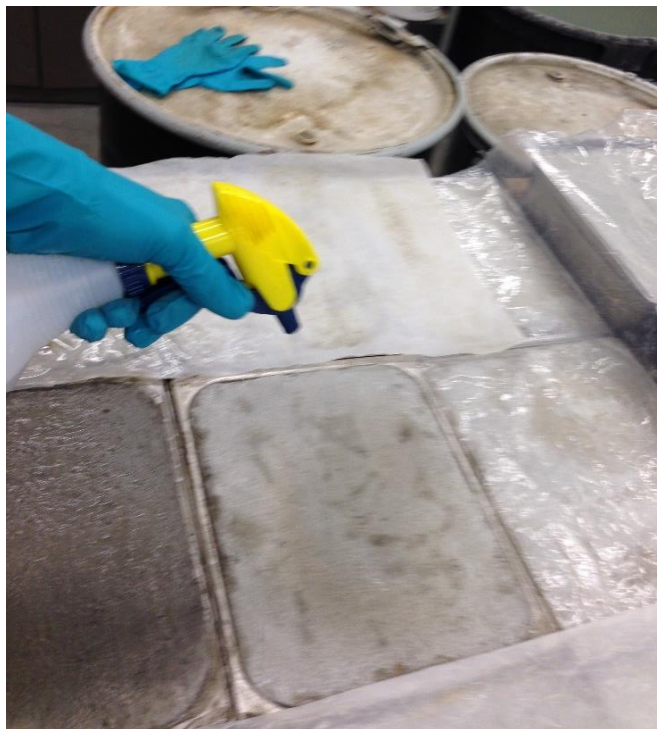
Figure 53. Sealer being sprayed and applied to concrete.
