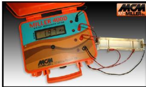
Figure 8. Miller 400D soil resistivity meter (M.C. Miller, 2010)
