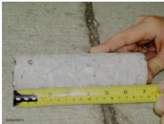
Core C-9: 7" long (broken)
