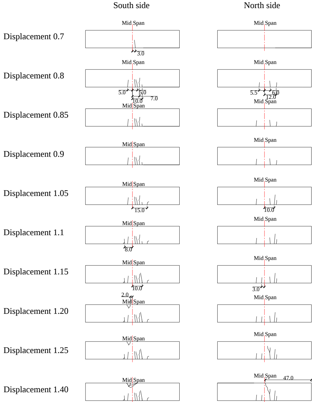
Figure C- 93 Panel CFRPT-NC-FL: Propagation of Cracking
