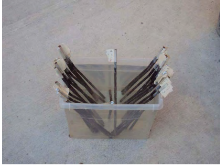
Figure C- 112 Steel Tendons Immersed in Muriatic Acid Solution
