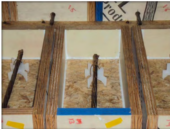
Figure C- 2 Non-Prestressed Corrosion Specimen - Formwork and Reinforcement
