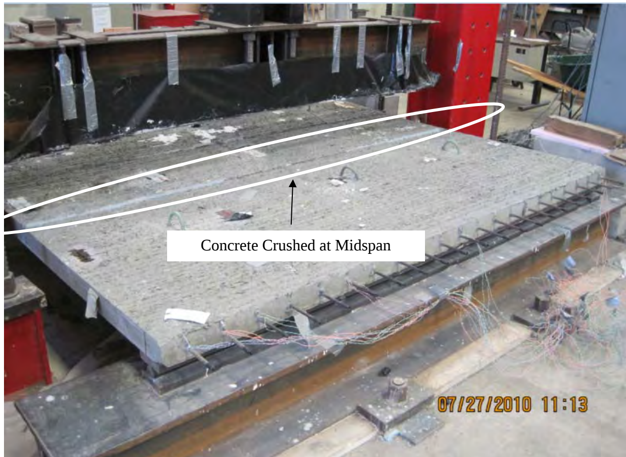
Figure C- 101 Flexural Failure at Midspan by Concrete Crushing of Panel CFRPT-FRC-FL
