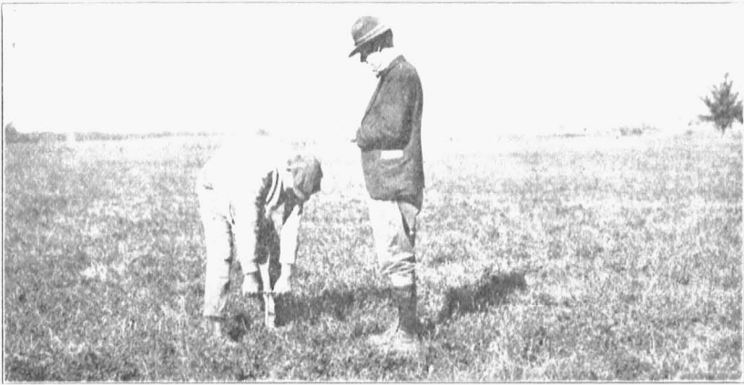
Fig. 2.—Soil survey inspectors at work; drawing a sample so that they may examine it. Borings are made to a depth of three feet.
