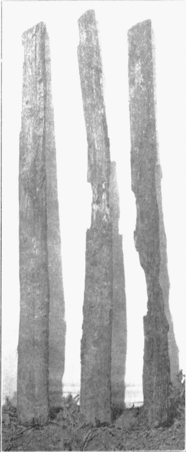
Fig. 3.—Variously treated white oak posts, after ten years in the ground (1) 5-hr. double tank-treatment of creosote; (2) 2-hr. double tank-treatment of creosote; (3) no treatment.
