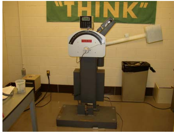
Figure 5.2 Tinius Olsen Model 84 Universal Impact Tester
