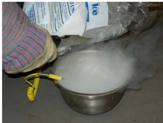
Figure 5.3 Dry-Ice and Alcohol Bath
