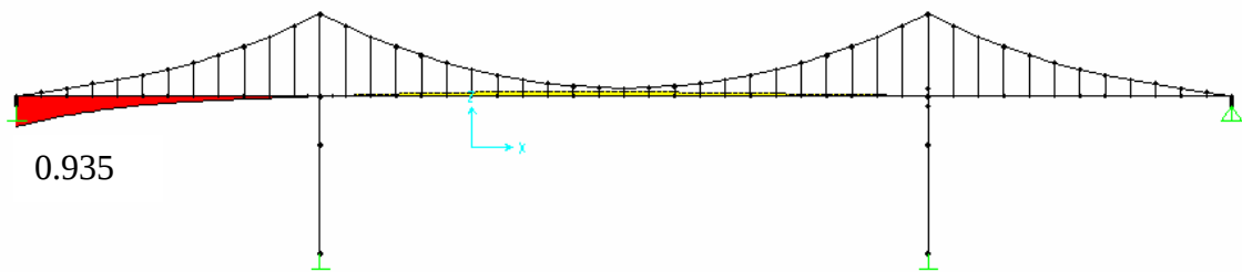
Figure E.2 Lane 2 Southeastern Strut Axial Load Influence Line
