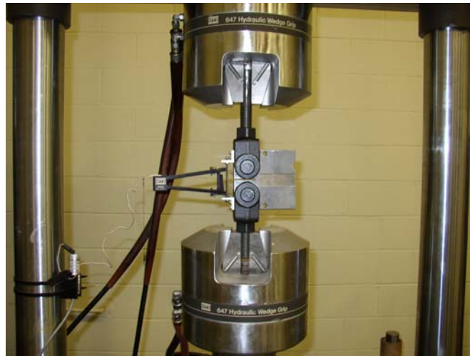
Figure 6.4 Crack Growth Test Set-up
