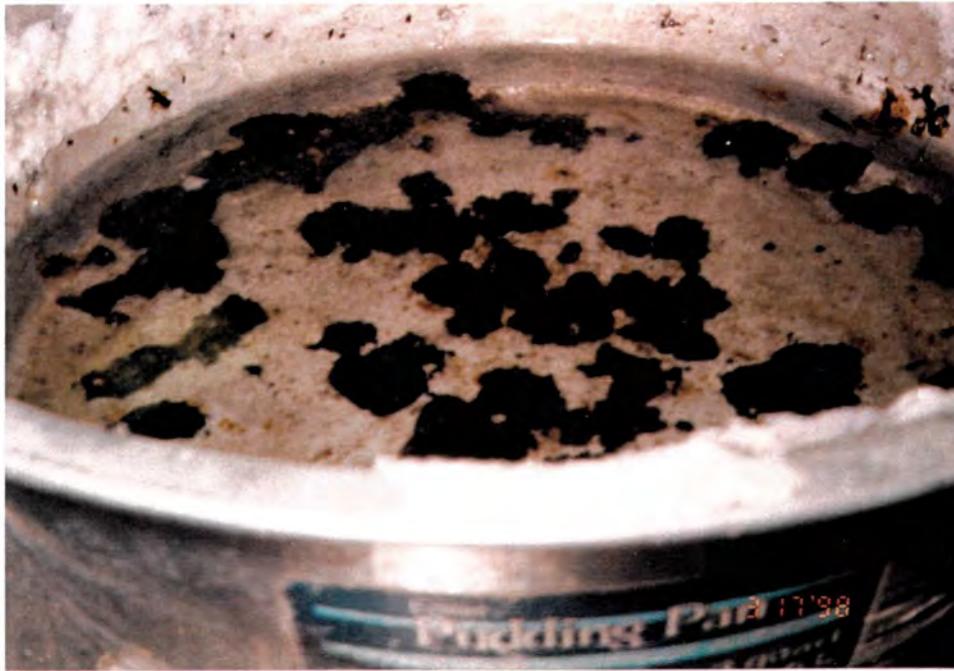
Photo #1: Samples of the seal soaking in salt brine. Oily clumps of the emulsion were floating on the surface and can be seen on the sides of the container. March 17, 1998; District 1, Andrew County Business Route 71
