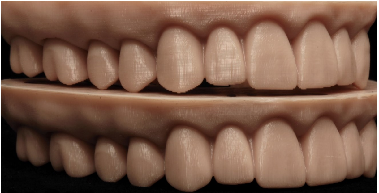
Figure 7. Experimental model print layer thicknesses. Experimental models printed with a layer thickness of 170 \mu\text{m} (above) and 100 \mu\text{m} (below) at a build angle of 0^\circ .
