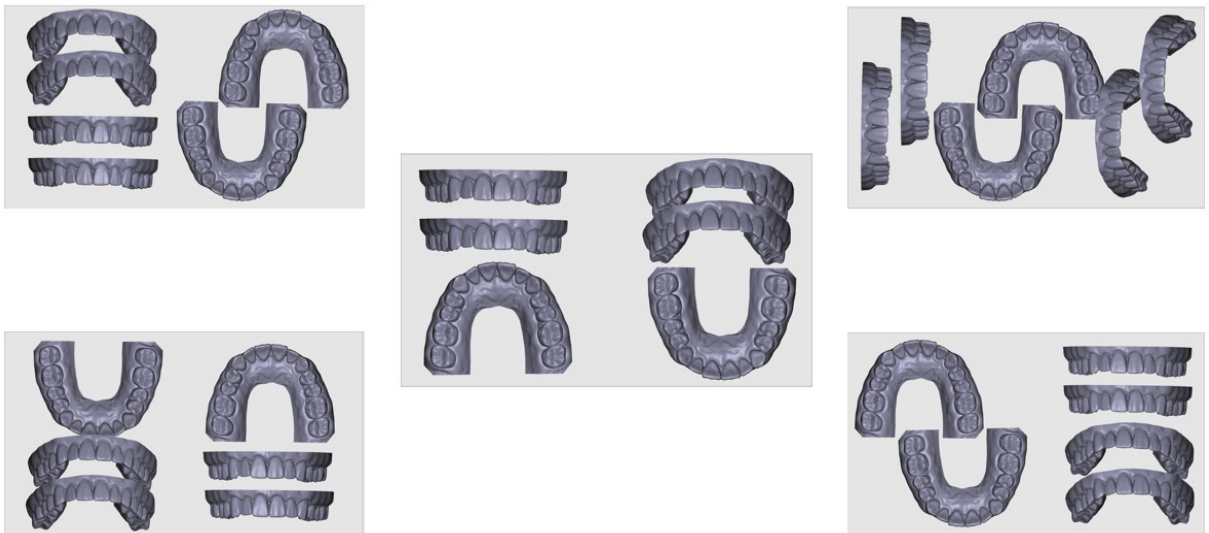
Figure 8. Experimental model print batches. Each of the five print batch arrangements with three build angles and two models per build angle.
