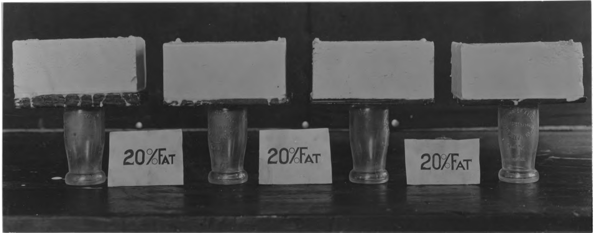
Fig. XIV. Original Brick before Exposure to Summer Temperature of 30°C.
