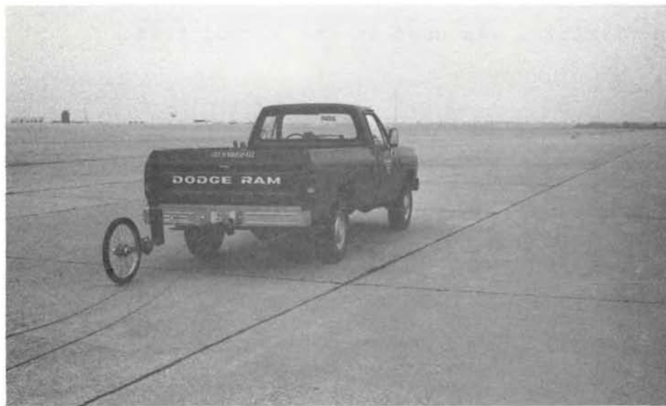
Figure 3. Cable Guidance System and Tow Vehicle
