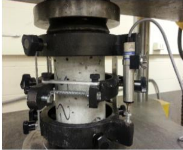
Figure 4-9. Modulus of elasticity test setup
