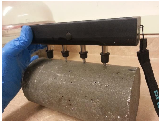
Figure 4-12. Surface resistivity measurement
