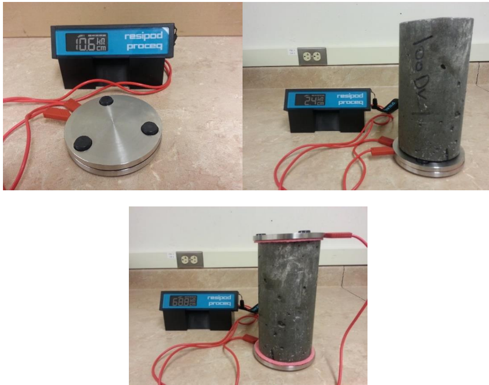
Figure 4-14. Measuring bulk electrical resistivity
