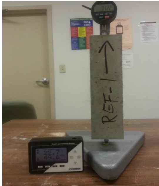
Figure 4-1. Photo of length measurement for drying shrinkage
