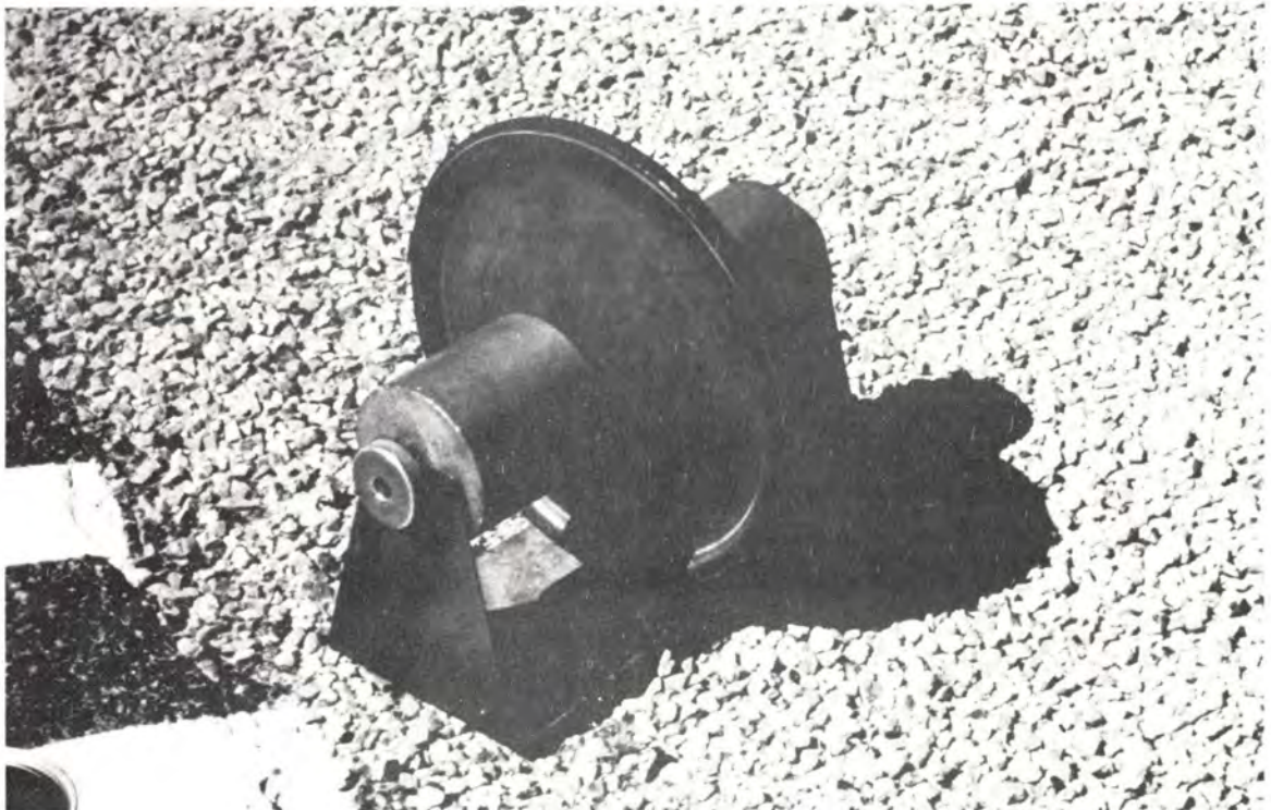
Figure 4 - Dry Time Wheel and Weight Assembly
