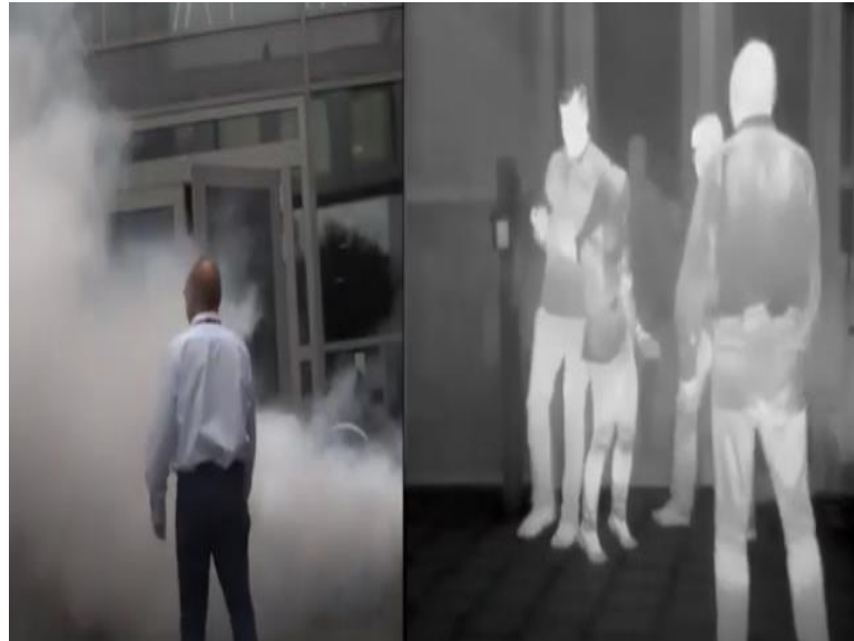
Figure 1.2: Temperature detection in smoky environment using infrared detectors.
