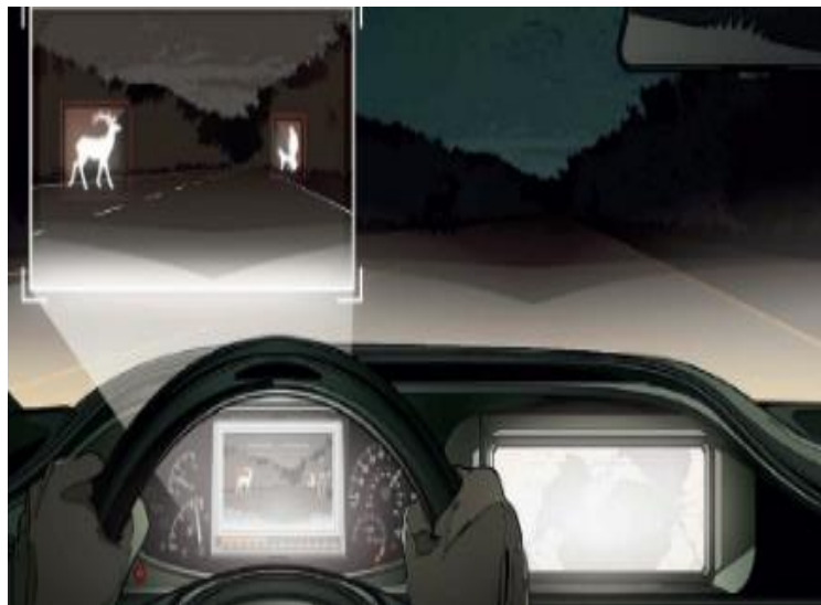
Figure 1.1: Thermal imaging makes night driving clearer and help avoiding accidents.
