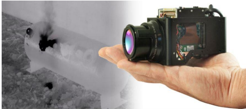
Figure 1.8: Gas leak detection using multispectral thermal imaging.
