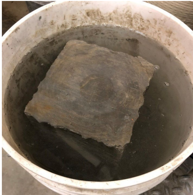
Figure 3-10 Wet specimen being soaked for 3 weeks
