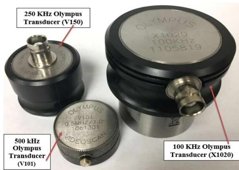
Figure 3-3 Pressure wave transducers used for testing [20]
