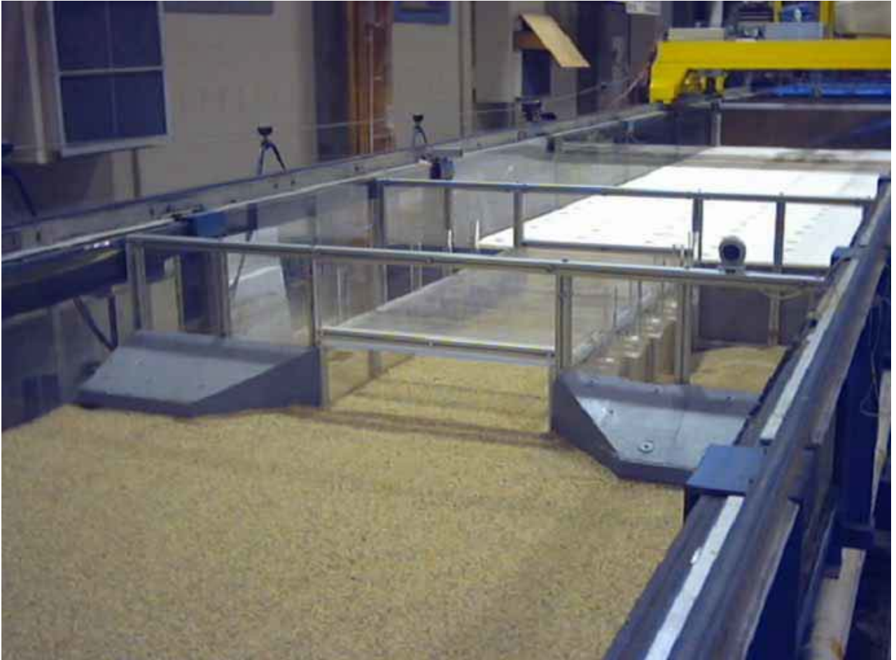
Figure 3. Culvert Model (FHWA 2003)
