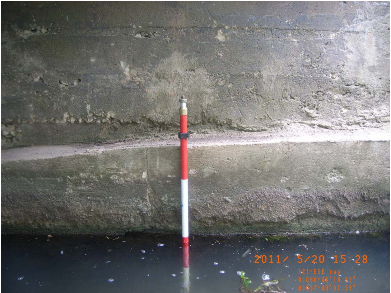
Figure 7 – Standard Scour Measurement Tool
