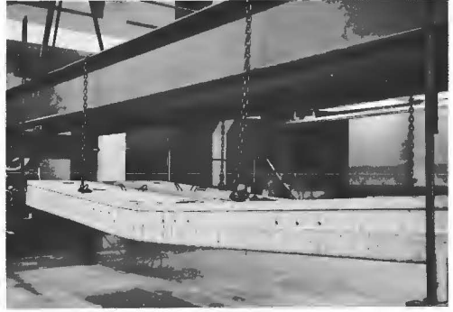
Figure 24. Crack pattern at ultimate load.
