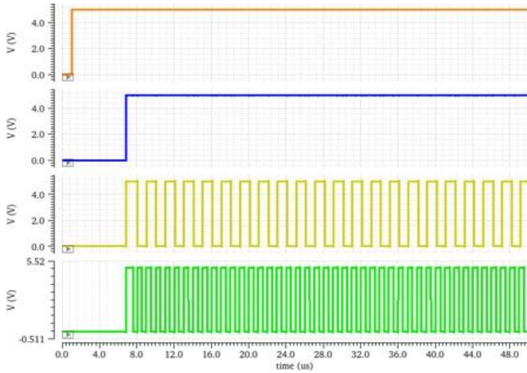
Figure 5.5: Transient analysis of the oscillator.
