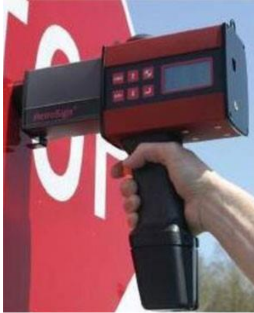
Figure 3. Retroreflectometer Traffic Sign Inspection (FHWA 2018)
