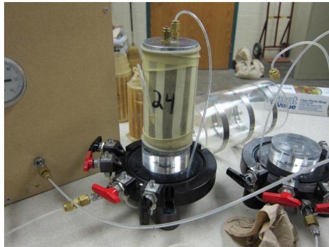
Figure 3.15 Specimen after testing placed in pressurized triaxial cell
