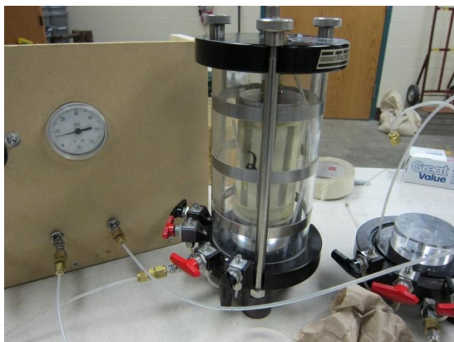
Figure 3.16 Specimen confined in pressurized cell
