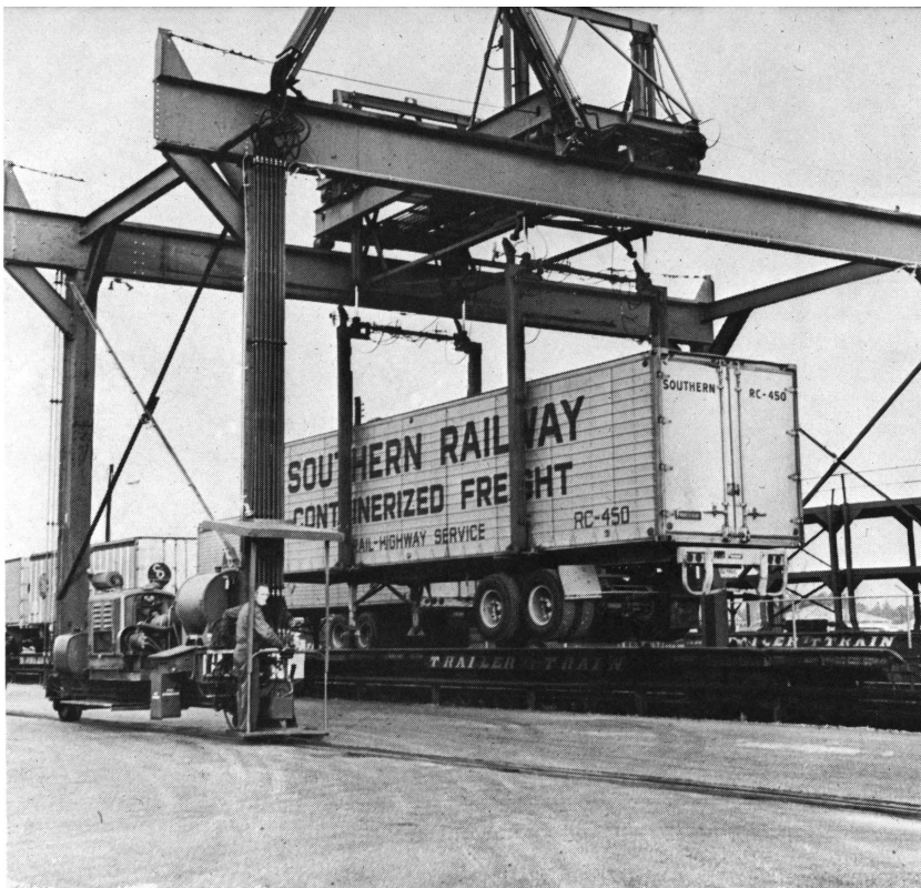
Truck-trailer being lifted from flatcar in piggyback operation. —Southern Railway System photo
