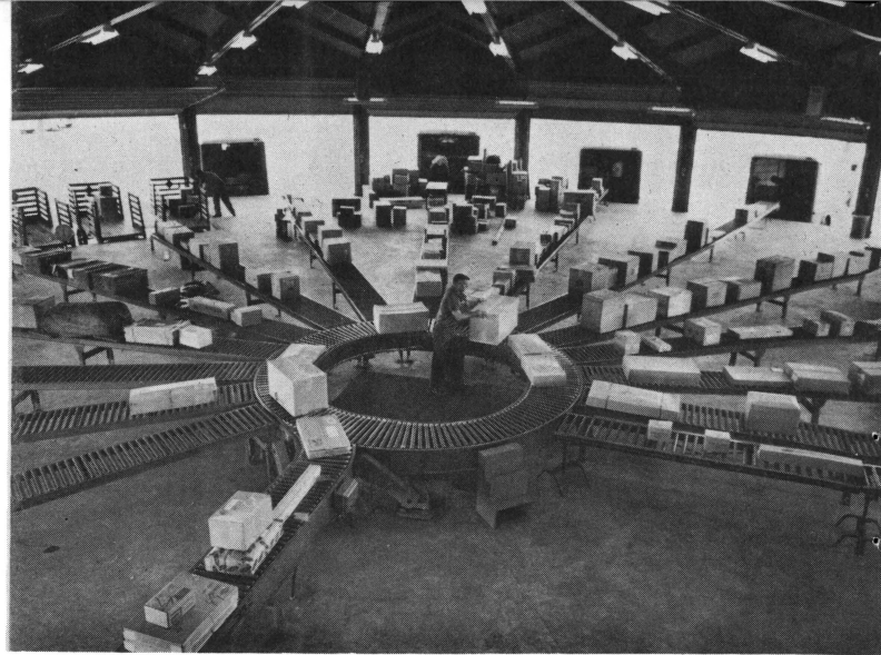
New REA Express key-point terminal at Savannah, Ga., features unique radial conveyor system. —REA Express photo
