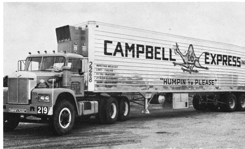
Closeup view of a refrigerated highway trailer. Notice underslung and front-mounted reefer units. — Campbell 66 Express photo
