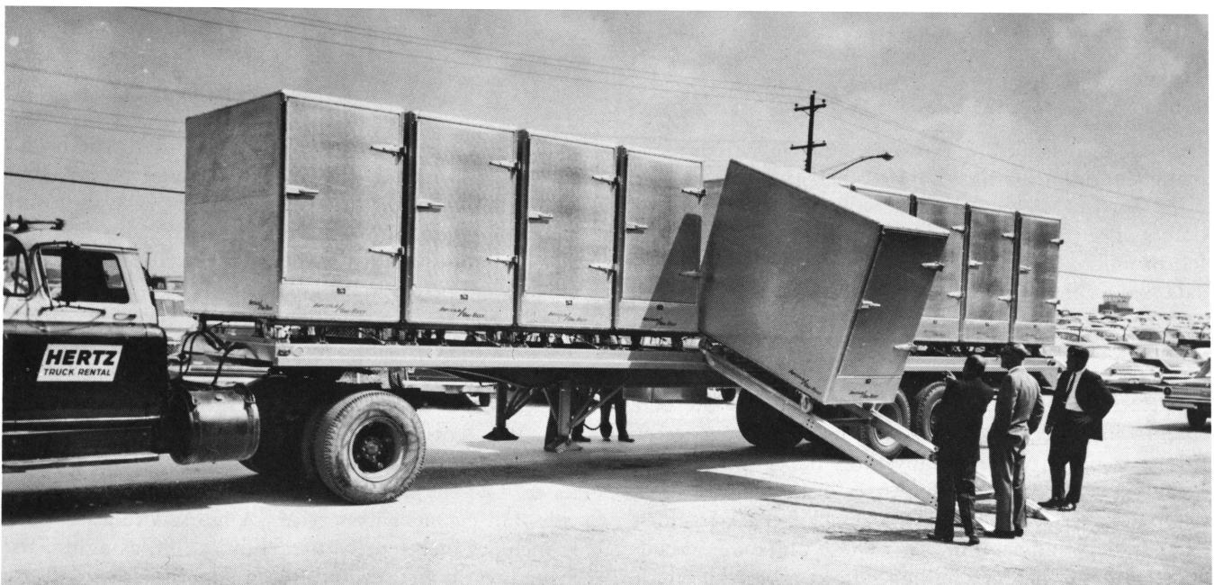
Another container system for transporting temperature-sensitive foods over long distances without mechanical refrigeration. Containers may be loaded or unloaded by one man with ramp and winch. —AVCO Corp. photo
