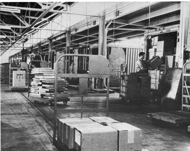
A drag-line operation in a modern truck terminal. — American Trucking Assns. photo
