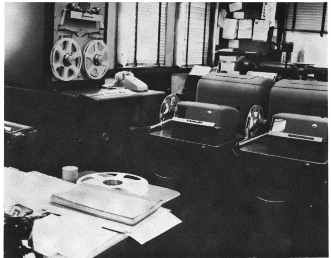
Machines in this communications center receive train consist information and punch the data on paper tapes for transmission. —Illinois Central Railroad photo
