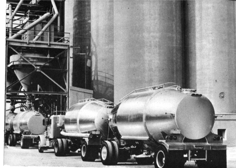
Aluminum hopper pressure tank-trains developed for handling bulk liquid commodities. —Fruehauf Trailer Co. photo
