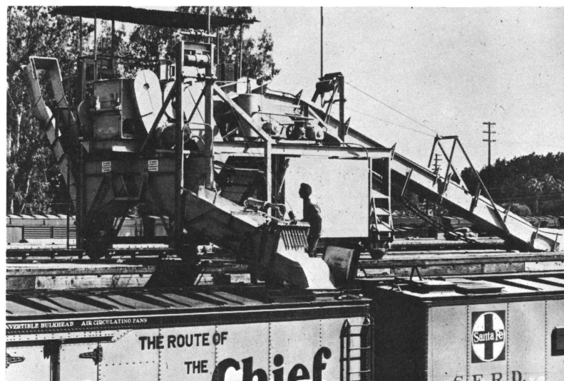
This electronically-controlled icing machine can ice a car in 90 seconds. —Santa Fe Railway photo
