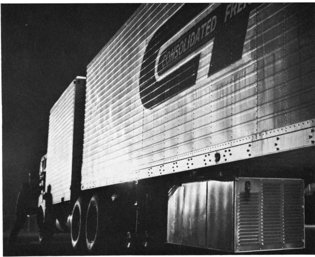
Night reefer schedule ready to hit the road, a 40-foot western insulated trailer with dromedary box and underslung refrigeration unit. —Consolidated Freightways photo
