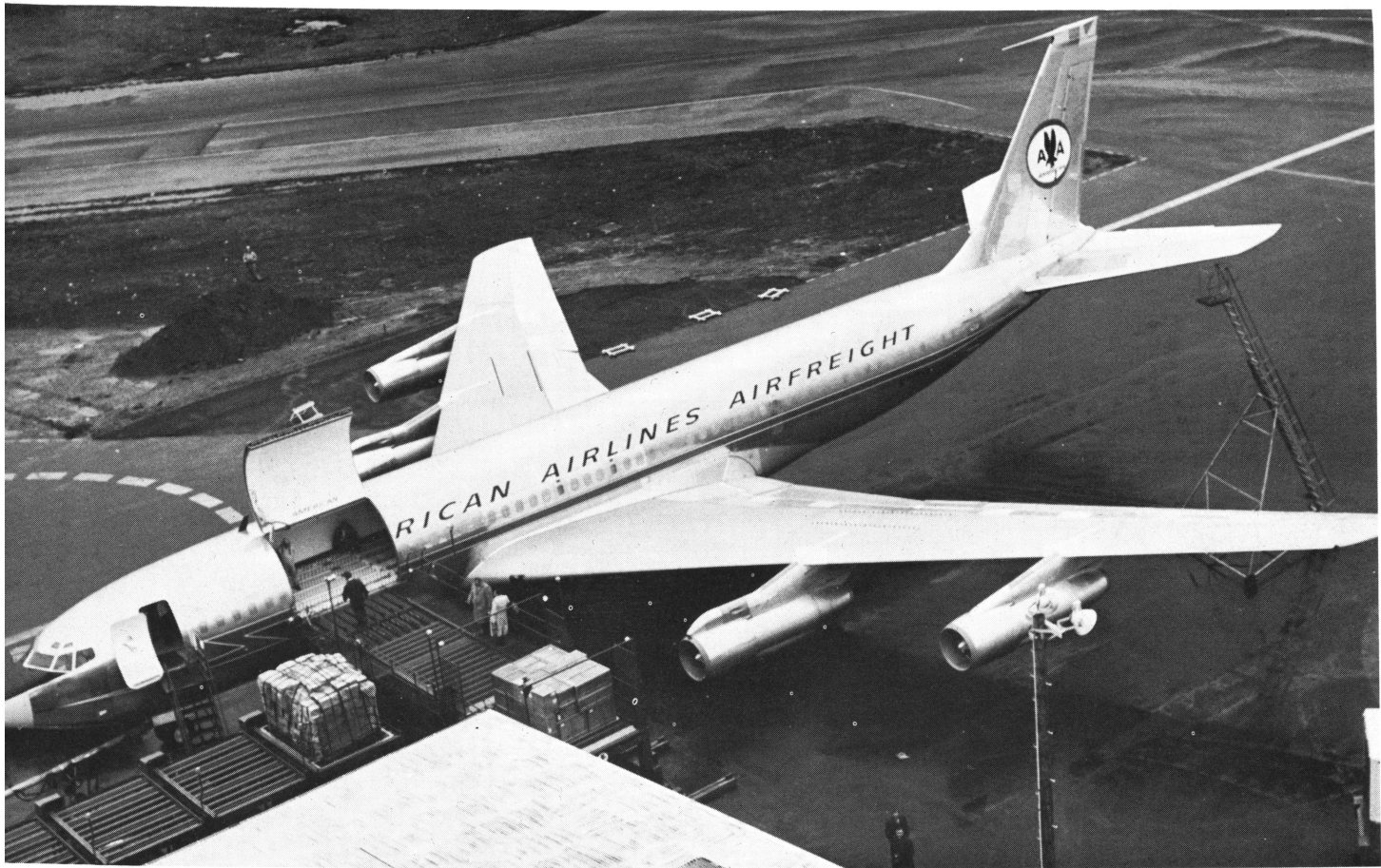
Cargo pallets are put aboard freight jets by mechanized loaders. These planes, which can carry 45 tons at up to
