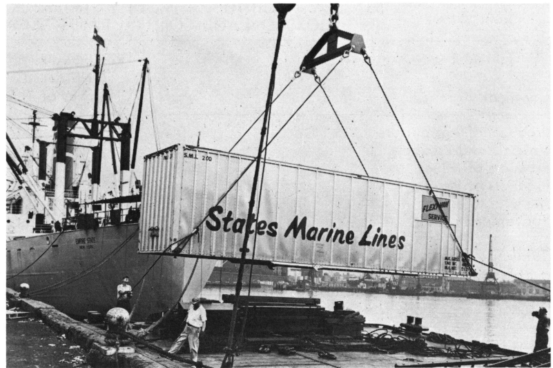
Sea-going container is lifted to deck of ocean vessel in New York Harbor for shipment overseas. —New York Central Railroad photo
