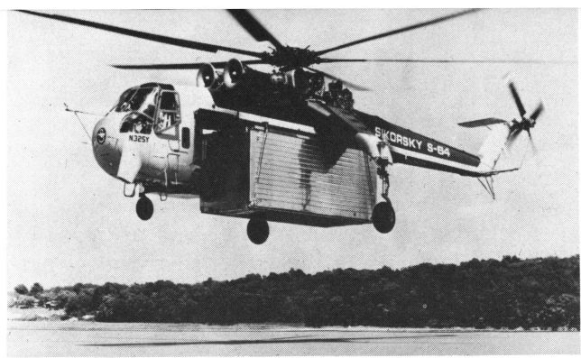
Twenty-foot aluminum container undergoes flight and lifting tests with Sikorsky Skycrane Helicopter. —Fruehauf Trailer Co. photo
