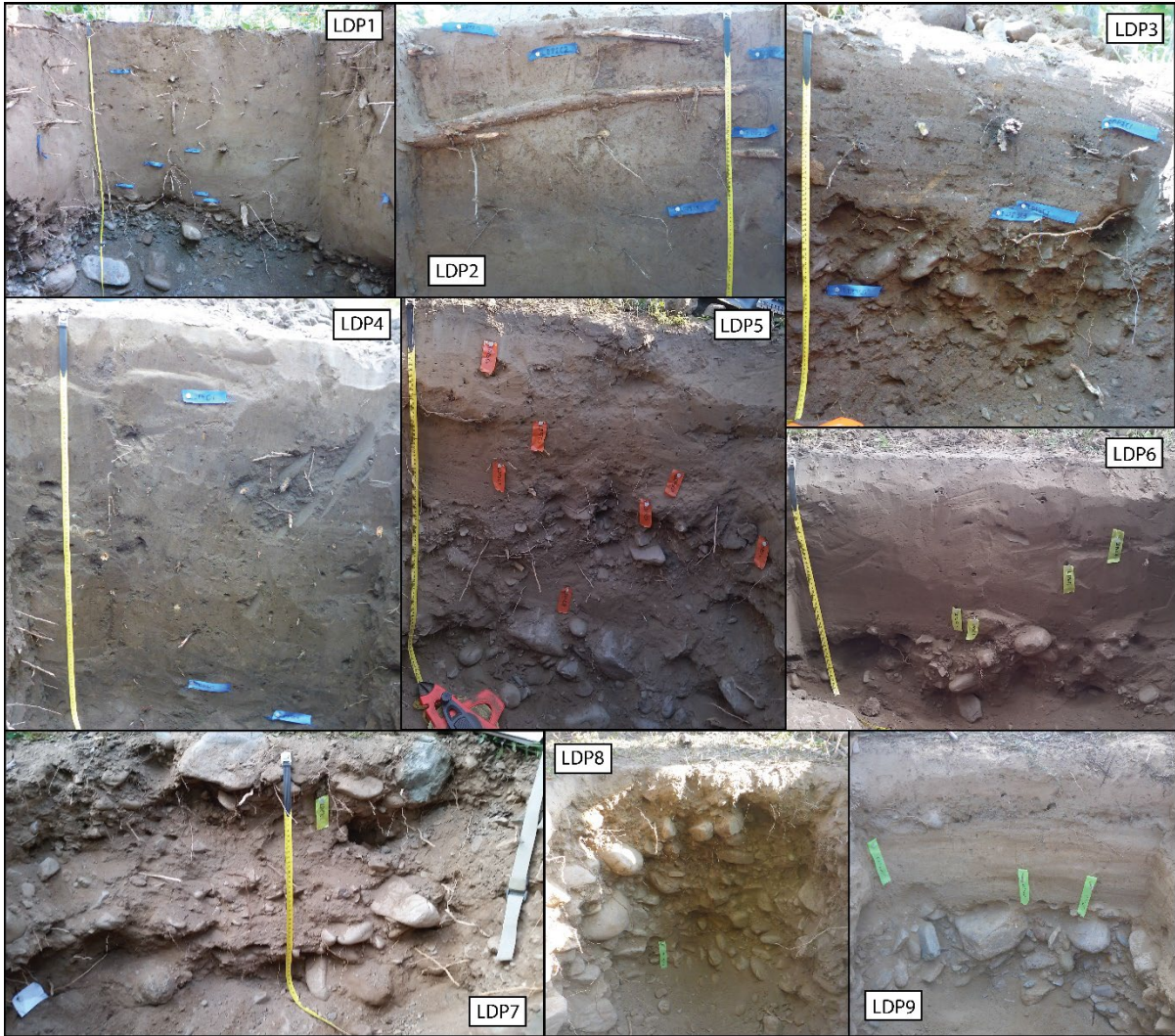
Figure 4.6: Terrace pit stratigraphy at Lal Dhang. Photographs of pits excavated on terraces adjacent to the Rawasan River show the stratigraphy of these surfaces. Detrital charcoal collection locations are tagged. Radiocarbon dates associated with these samples can be found in Figure 4.7.
