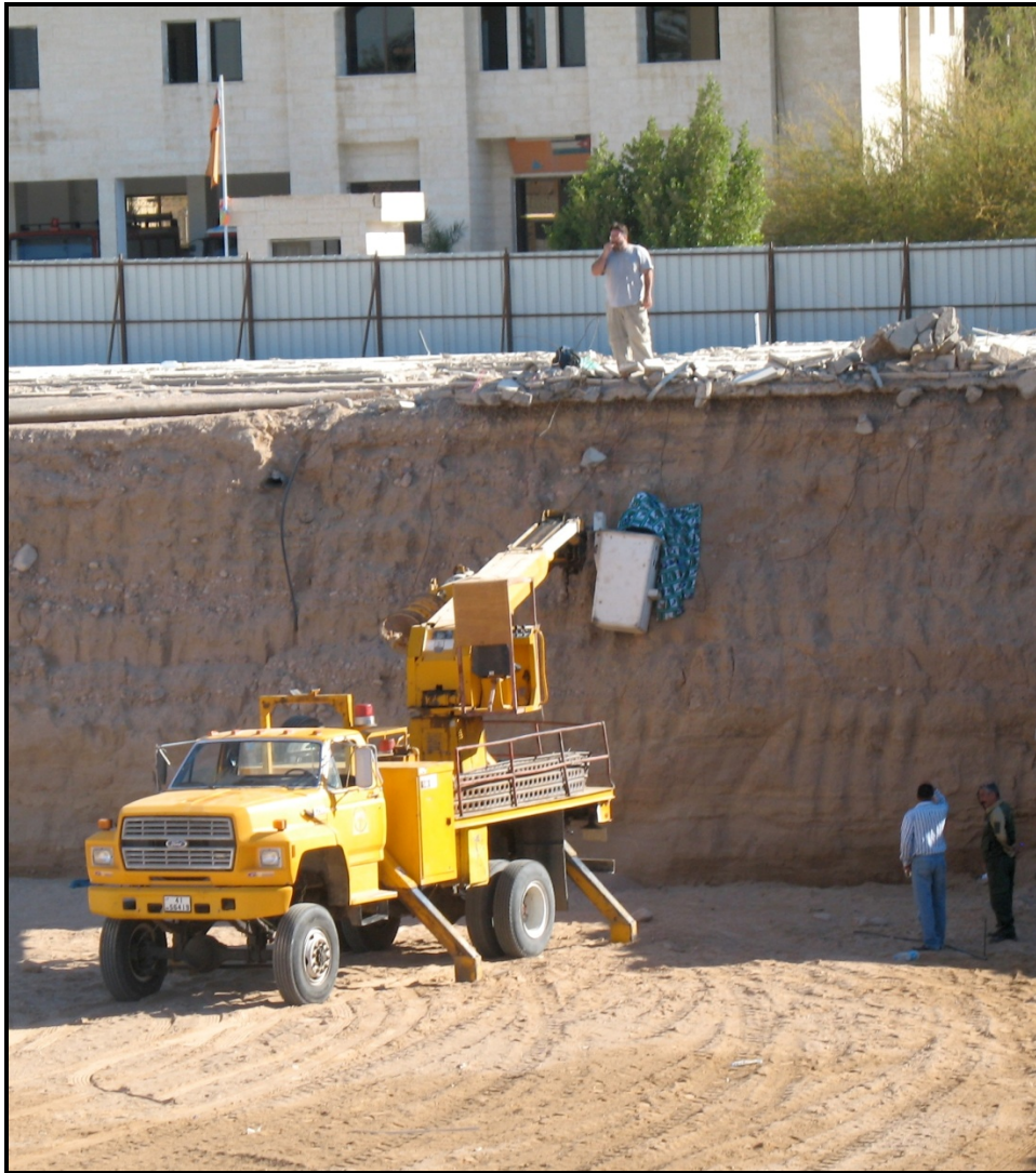
Figure 5.5 Collecting sediment samples to be dated using optically stimulated luminescence (OSL) along the southwest trench wall using a bucket truck supplied by the Department of Antiquities in Aqaba, Jordan. OSL samples were collected from beneath layers of dark sheets to avoid contamination (bleaching of sediment grains) by exposure to sunlight.
