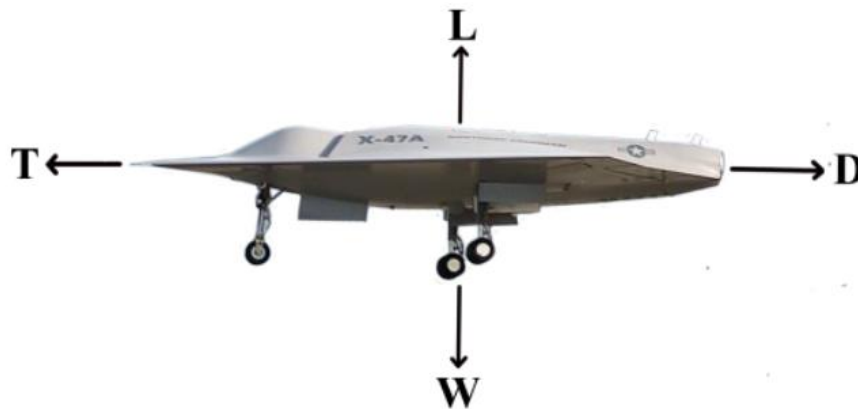
Fig. 2.2 Four Forces Acting on X-47A for SLUF
