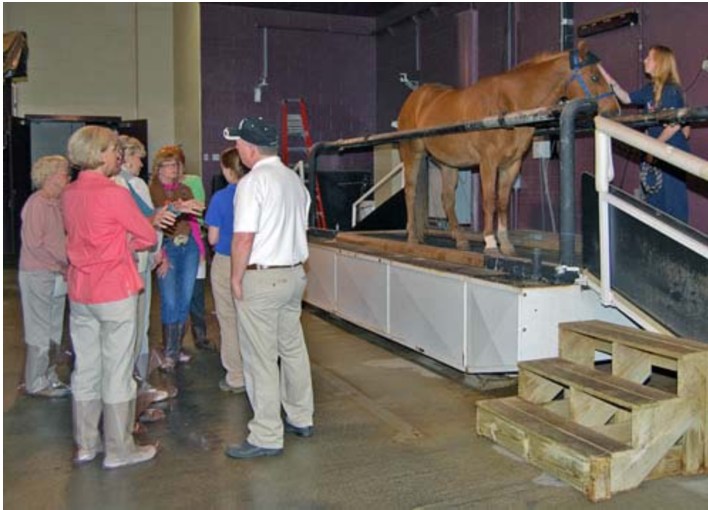
Saddle and Sirloin Club members also had the opportunity to see an equine treadmill. The treadmill is used to help pinpoint the cause of lameness in horses being treated at in the VMTH equine clinic.
