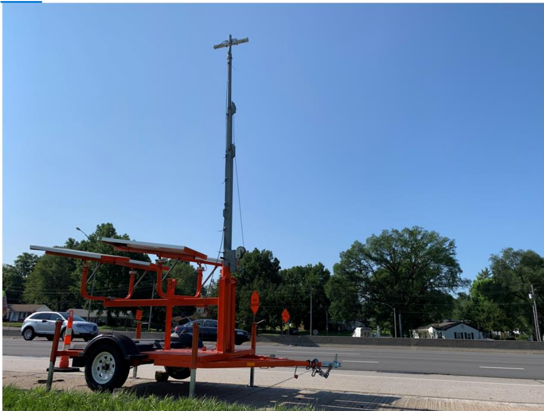
Figure 0-2. Trailer with SpeedLane® Pro sensor
