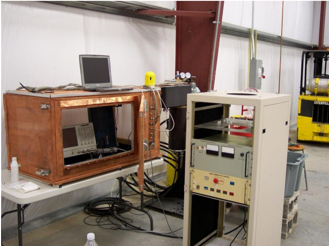
Figure 3. 5: A Picture of the control station, the Faraday cage, and the oscilloscope of the voltage breakdown test stand
