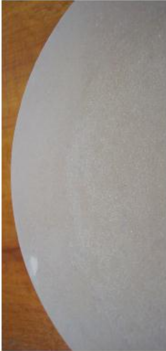
Figure 4.97: A picture of the surface of 75% filler by volume BST-PVDF composite
