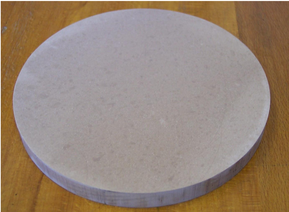
Figure 3. 1: An example of a mixed dielectric disk after machining and sanding. This disk has a matrix of PVDF polymer with 65% BST by volume
