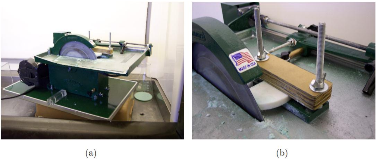
Figure 3. 2: The lapidary saw used in cutting thin slices of dielectric material. (a) shows the saw inside the fume hood and (b) shows the saw with a piece of the dielectric material that it was cutting
