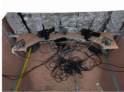
(b) Setup box interior as seen from the opening used to replace plant roots after imaging.
