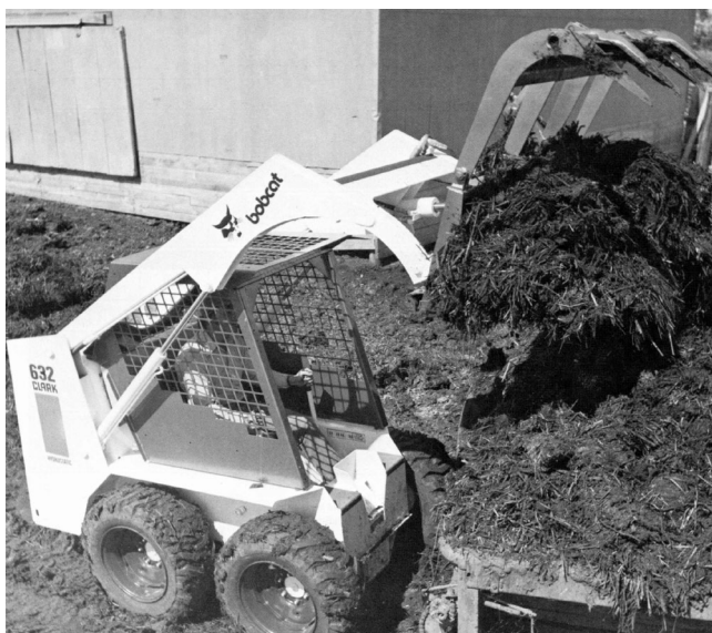
Figure 3. Front-end or skid steer loaders are necessary for handling bedding and manure in hoop structures.
