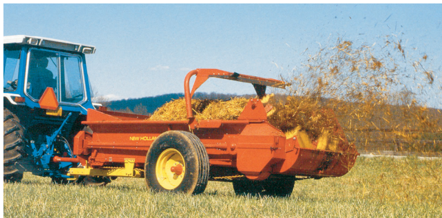
Figure 4. Manure spreaders should be able to handle stringy, fibrous mixtures of manure and bedding from hoop structures.
