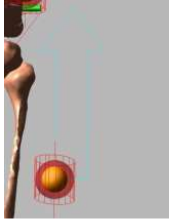
Figure 3.7. Motion constraints (yellow spheres) are attached to the body via a bushing. The red spheres illustrate the location of the marker on the body.
