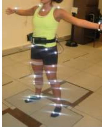
Figure 3.2. Subject poses in a static trial that will be later used to adjust the location of marker placements to the body segments.
