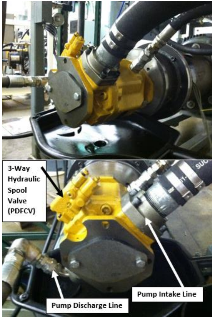
Fig. 3. LS pump and PDFCV (3-way hydraulic spool valve)
