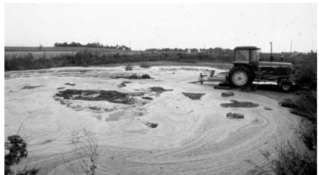
Figure 3. A propeller-type agitator can be used to resuspend settled solids (sludge) from the bottom of a lagoon during pump-down.
