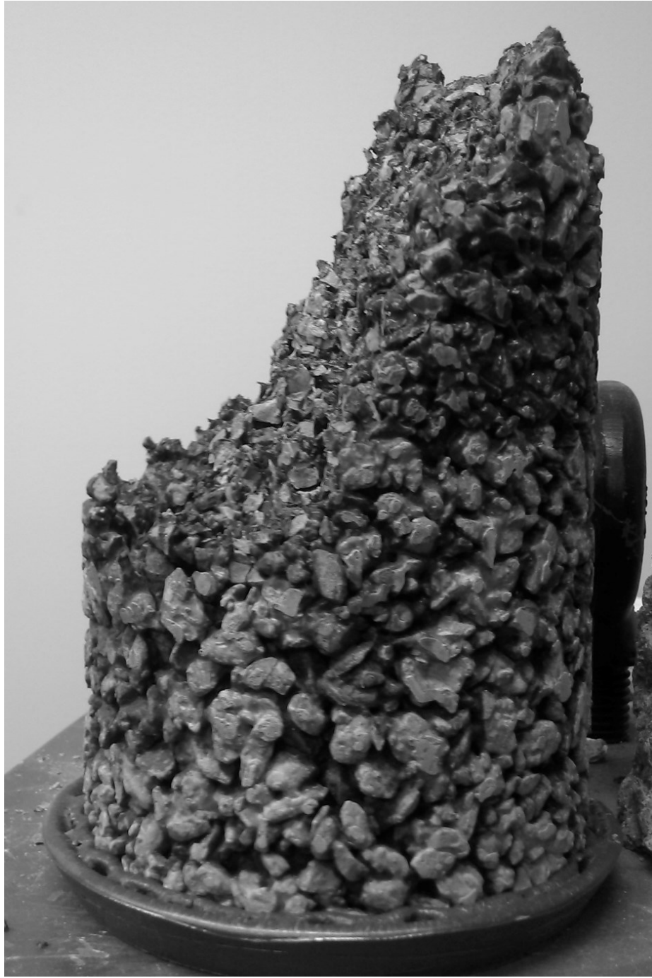
Figure 32 Typical Shear Mode of Failure After ASTM C39 Testing
