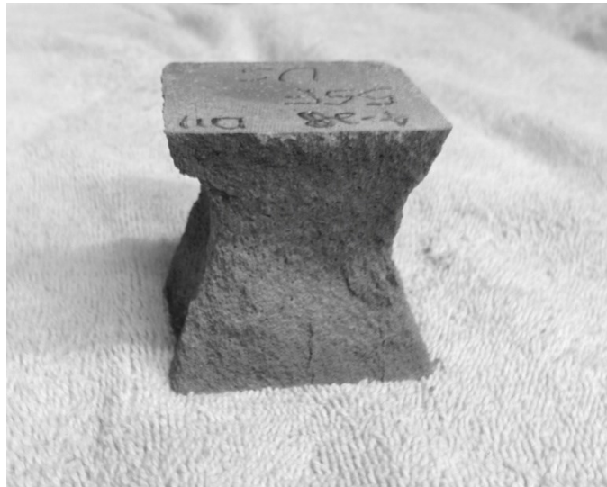
Figure 24 Typical Mortar Cube Failure
