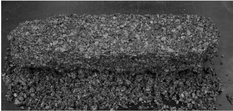
Figure 53 5-LS-25 After ASTM C666 Testing
