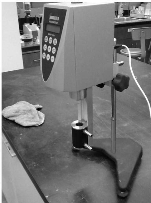
Figure 5 Brookfield Viscometer Model Used for Testing
