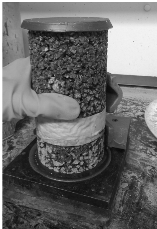
Figure 8 Capping-Capping Process for Compressive Strength Testing
