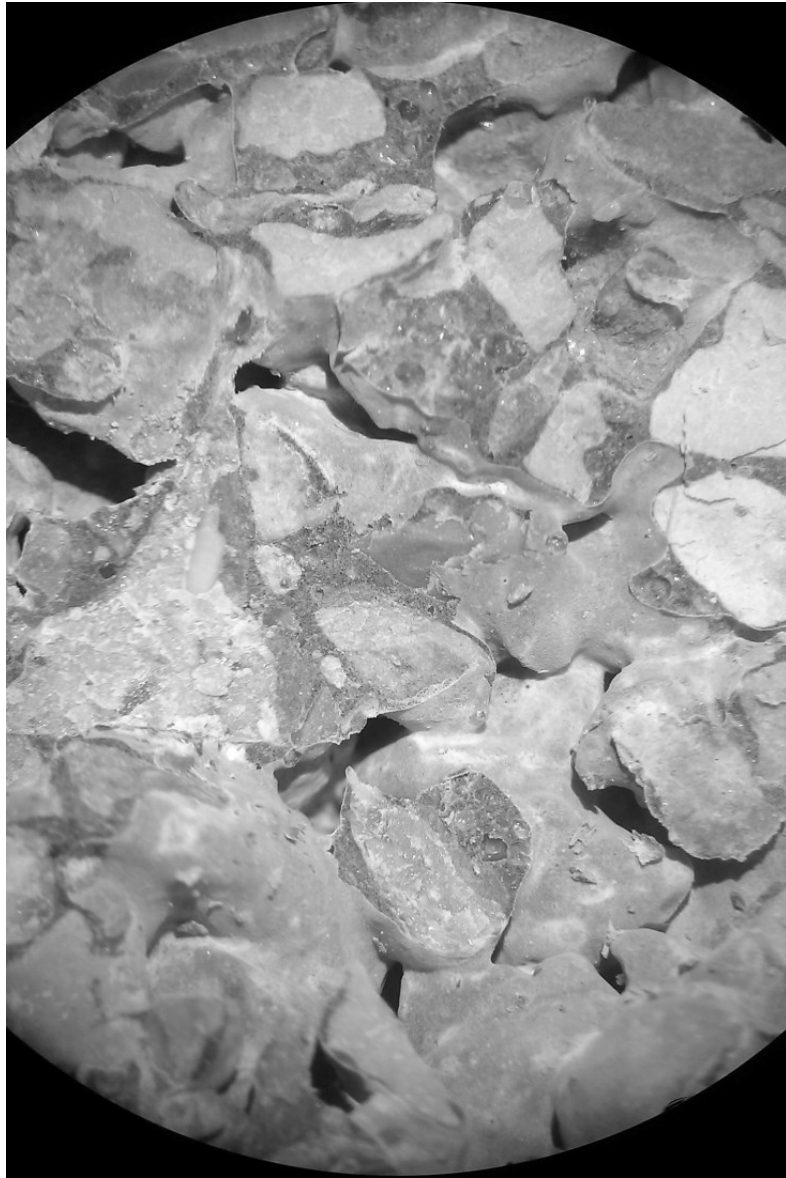
Figure 35 Aggregate Fracture in 5% SF Sample
