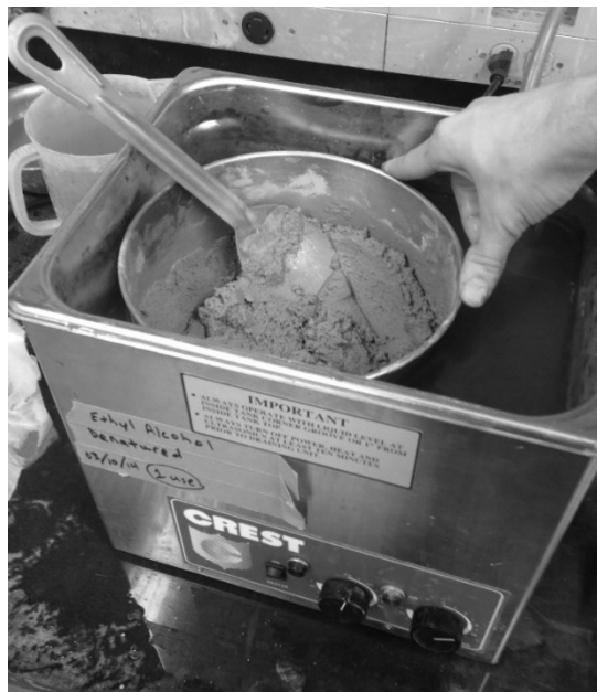
Figure 3 Mortar Ultrasound Mixing
