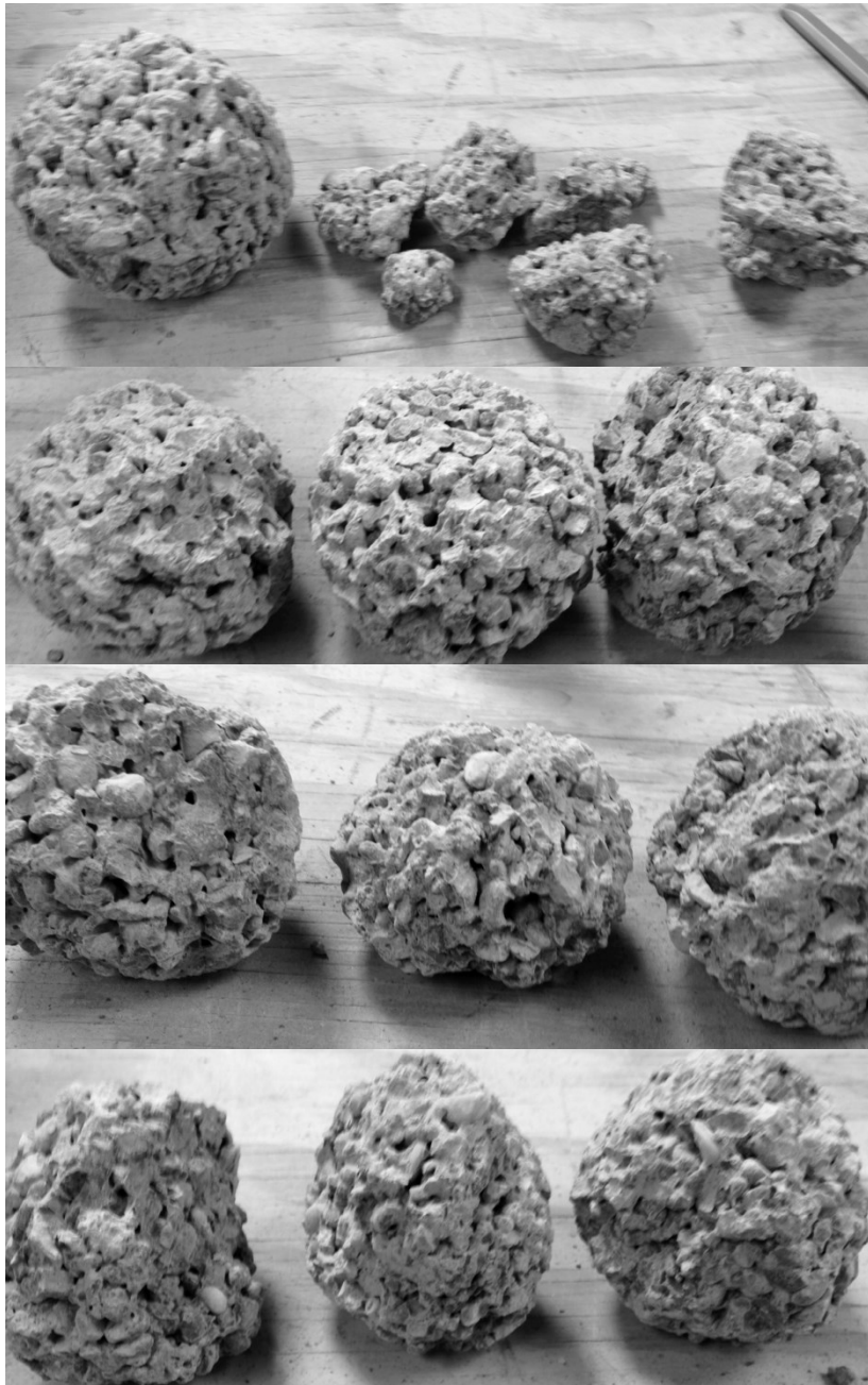
Figure 47 River Gravel Samples After Impact Abrasion by ASTM C1747 from Top to Bottom 0-RG-20, 5-RG-20, 0-URG-20, 5-URG-20
