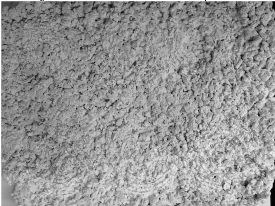
Figure 42 5-LS-20 ASTM C944 Abrasion Sample
