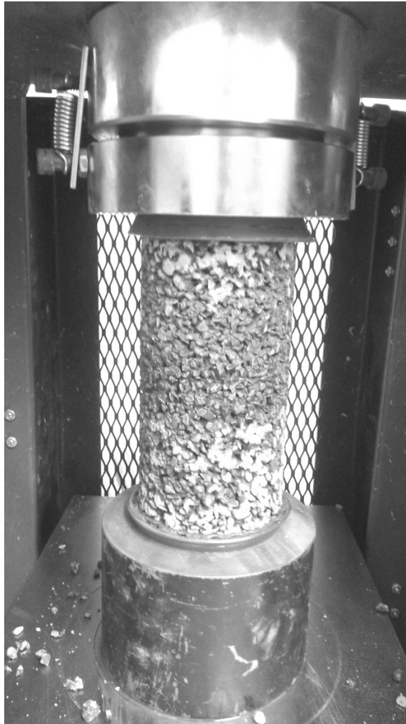
Figure 9 Compressive Strength Testing of a Pervious Concrete Sample.
