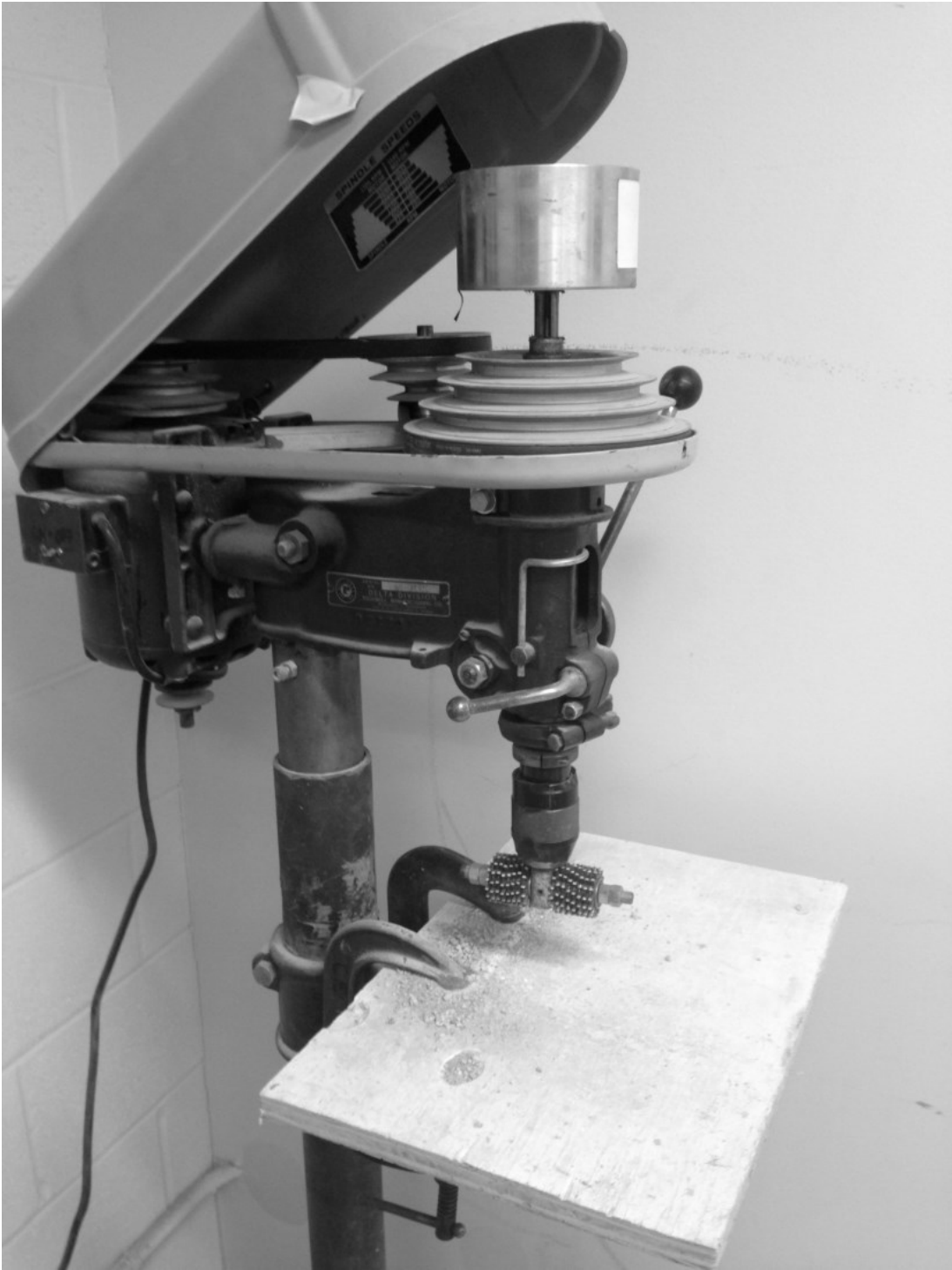
Figure 11 ASTM C944 Rotary Abrasion Apparatus
