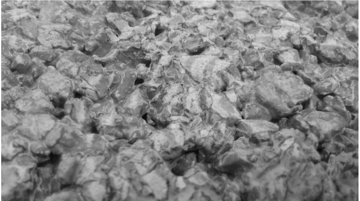
Figure 43 7-LS-20 ASTM C944 Abrasion Sample
