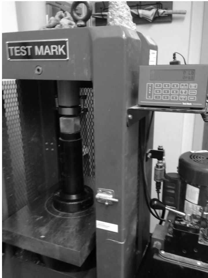
Figure 7 ASTM C109 Mortar Cube Compressive Strength Testing
