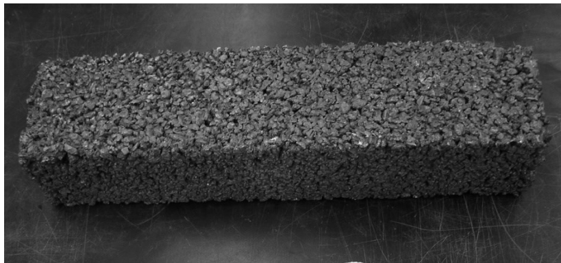
Figure 52 5-LS-25 Before ASTM C666 Testing
