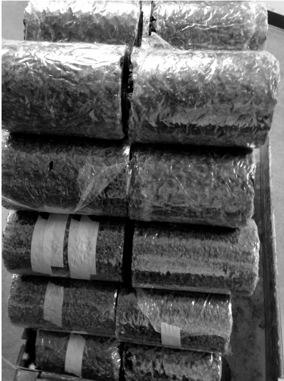
Figure 15 Pervious Concrete Permeability Test Samples
