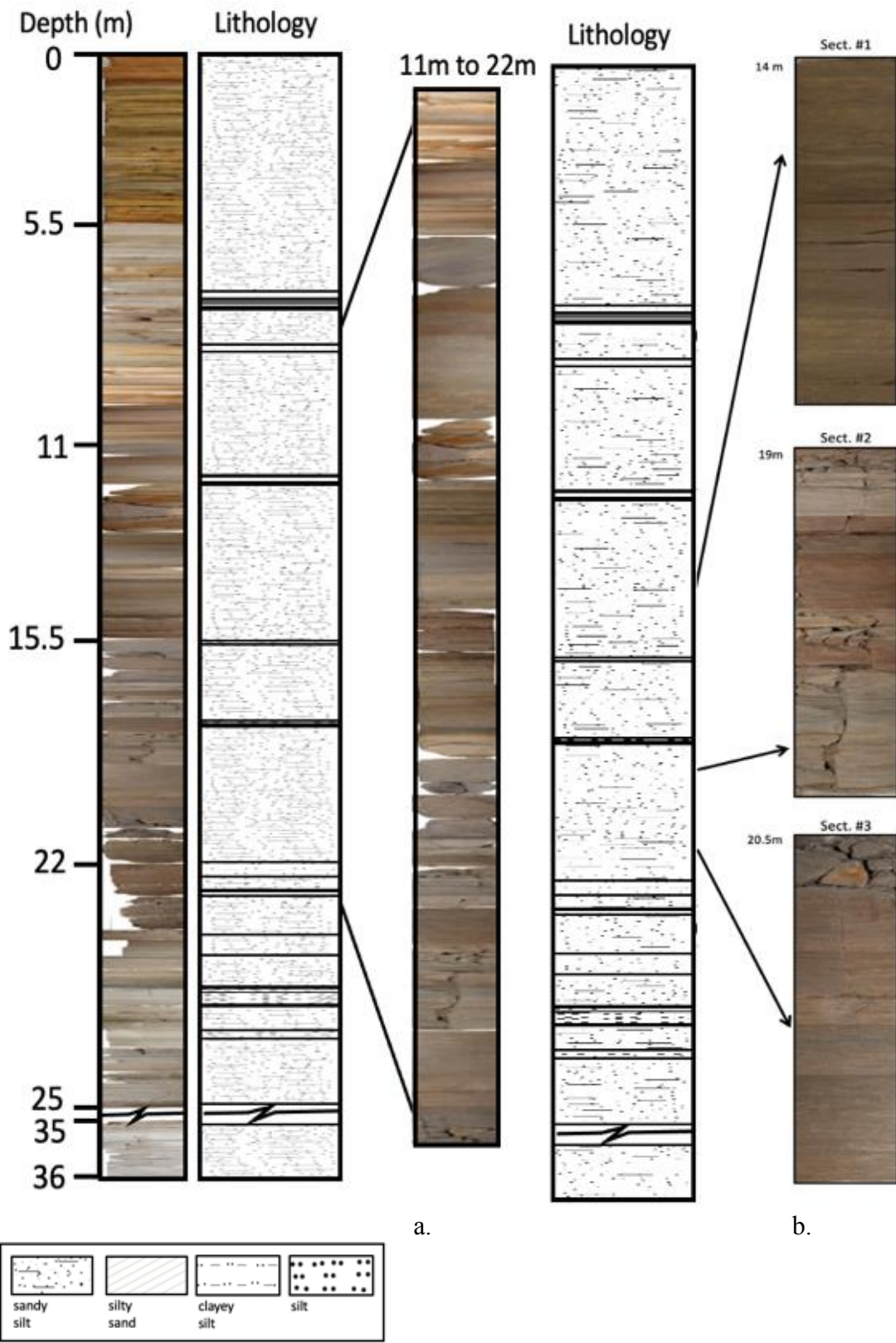
Figure 5.1. AZ2 cored sediments images, lithology, and legend. (a.) 11 m to 22 m exhibited laminated sediments; (b.) Section 1 (14 m to 14.50 m, Section 2 (19.00 m to 19.50 m), Section 3 (20.5 m to 22 m) analyzed for micro-facies.
