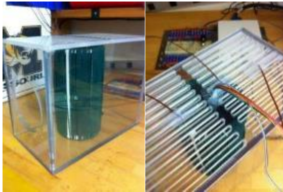
Figure 2-23 Scaffold with cotton threads in container
