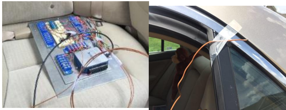
Figure 3-1 Data Acquisition System Connected with Sensors and Laptop and Sensor T1 position.
