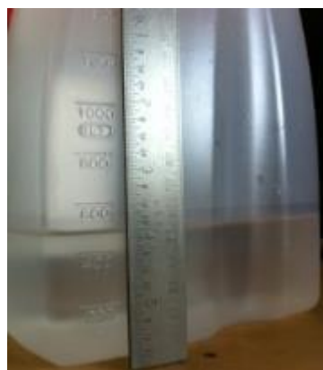
Figure 2-25 Measuring water level change
