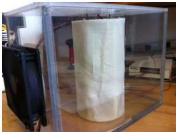
Figure 2-24 Pour water into container while the scaffold stands inside the water container
