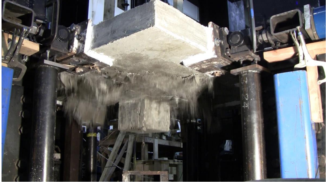
Figure 4.4.2.1 – Dynamic 3 test just after punching failure
