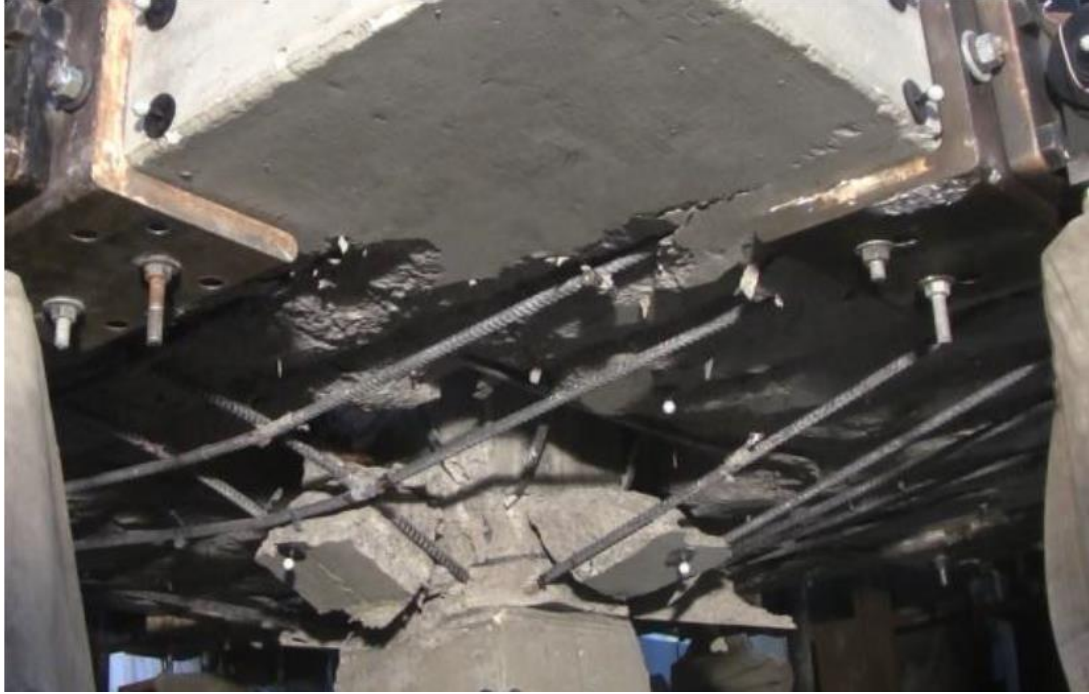
Figure 4.4.1.3 – Underside of the static 0.64% test at conclusion of testing
