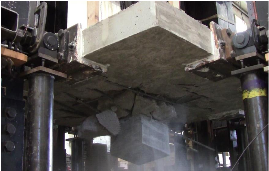
Figure 4.4.1.4 – Underside of the Dynamic 1 test at the conclusion of testing
