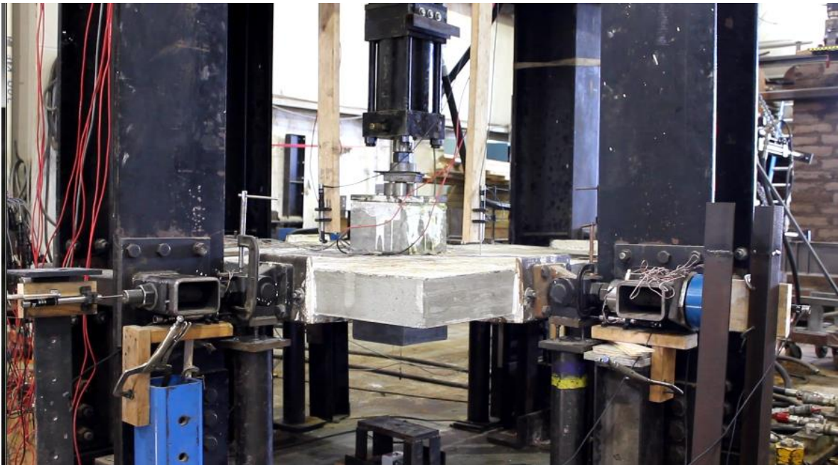
Figure 4.1 – Overall view of test setup and slab specimen
