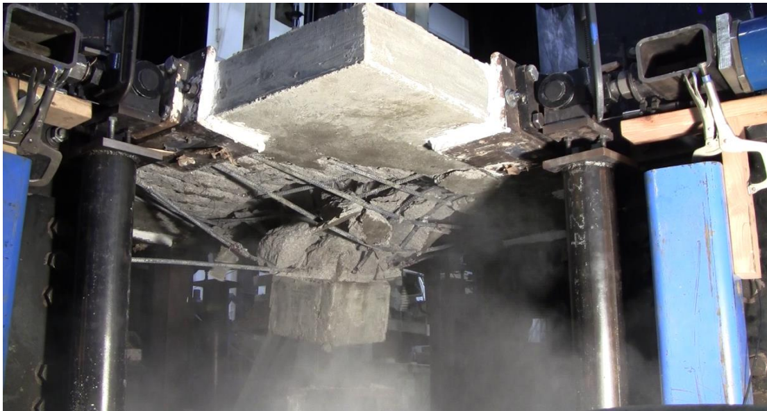
Figure 4.4.2.4 – Underside of the Dynamic 3 test at the conclusion of testing
