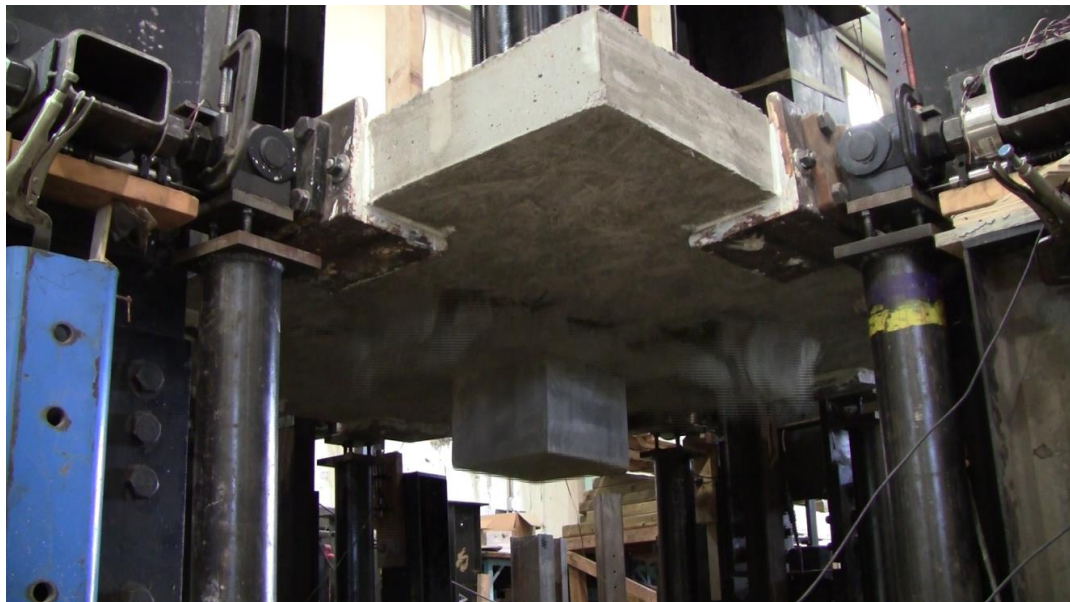
Figure 4.4.1.2 – Underside of the Dynamic 1 test at punching failure
