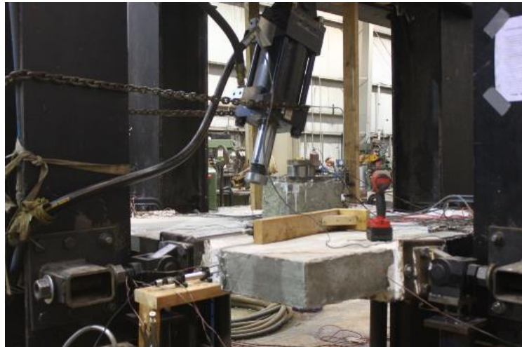
Figure 3.4.9 – Test setup with dynamic actuator, full ram displacement
