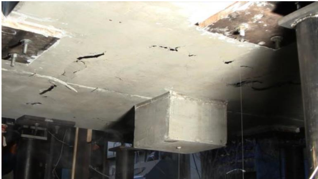
Figure 4.4.2.2 – Static 1.0% test just after punching failure
