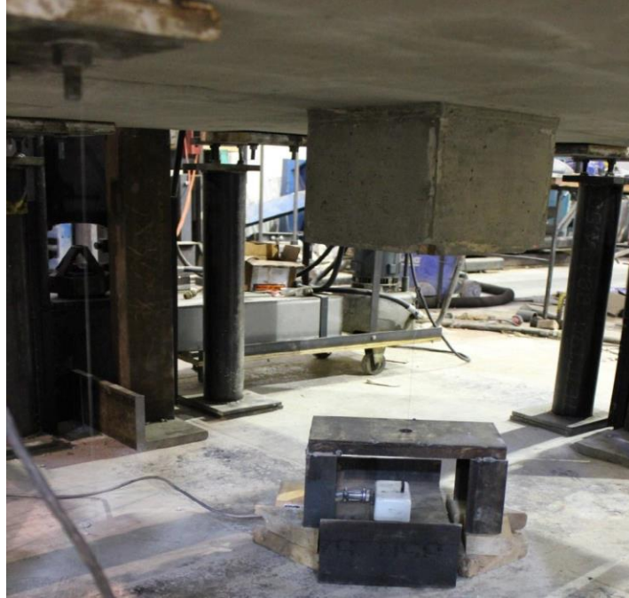
Figure 3.5.7 – String pot located directly beneath bottom column to measure deflection
