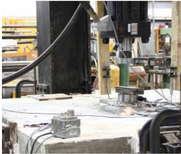
Figure 3.5.8 – Dynamically loaded test specimen after failure has occurred
