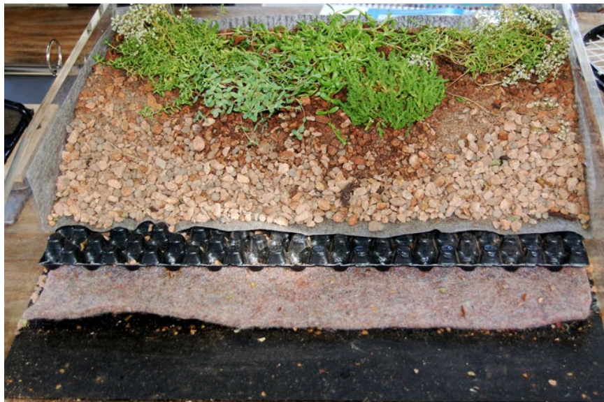
Figure 1.5: Vegetated Roof System Cross-Section (Wikipedia, 2006b)
