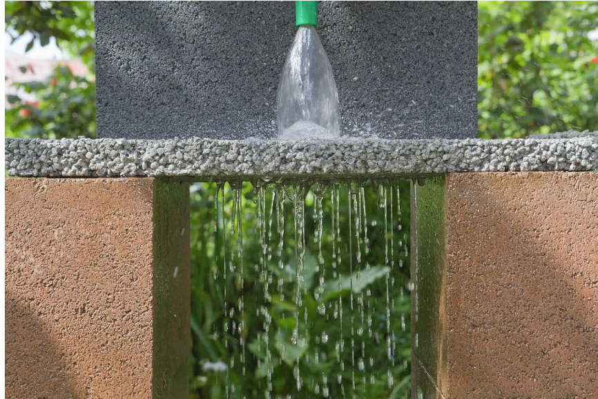
Figure 1.4: Permeable Pavement Example (Wikipedia, 2011)
