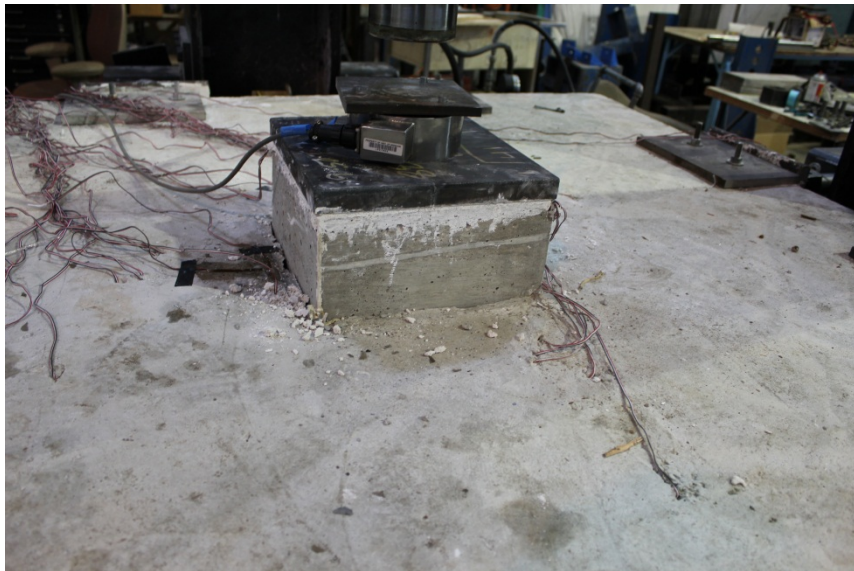
Figure A.12: Displaced top column stud after loading
