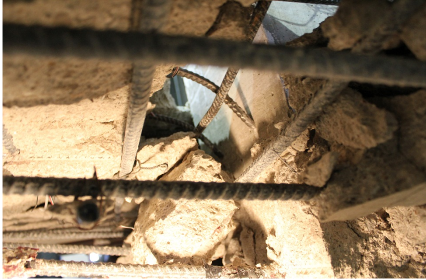
Figure A.11: Fracture #3 compression steel
