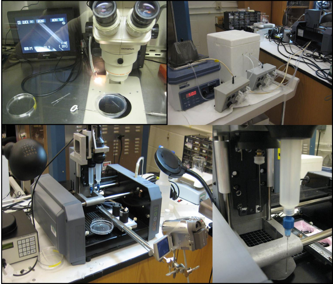
Figure 4. Manual and computer-aided tissue assembly system. Manual macro-tissue assembly was performed in a biological safety cabinet using video assistance ( top left ). Computer-aided assembly was performed using a specifically designed bioprinter ( bottom left ): the stage supports a Petri dish in which the tissue construct is printed, and two temperature-controlled chambers in which cold or hot water is circulated ( top right ); the printing heads consist of an extruder fitted with a syringe holding a glass micropipette with an inserted piston ( bottom right ).
