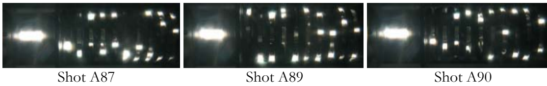
Fig. 9-28. \pm 45 kV, 35 psig, SF 6 6.67 cm, laser trigger. Ten cascade gaps visible, trigger gap at left.
