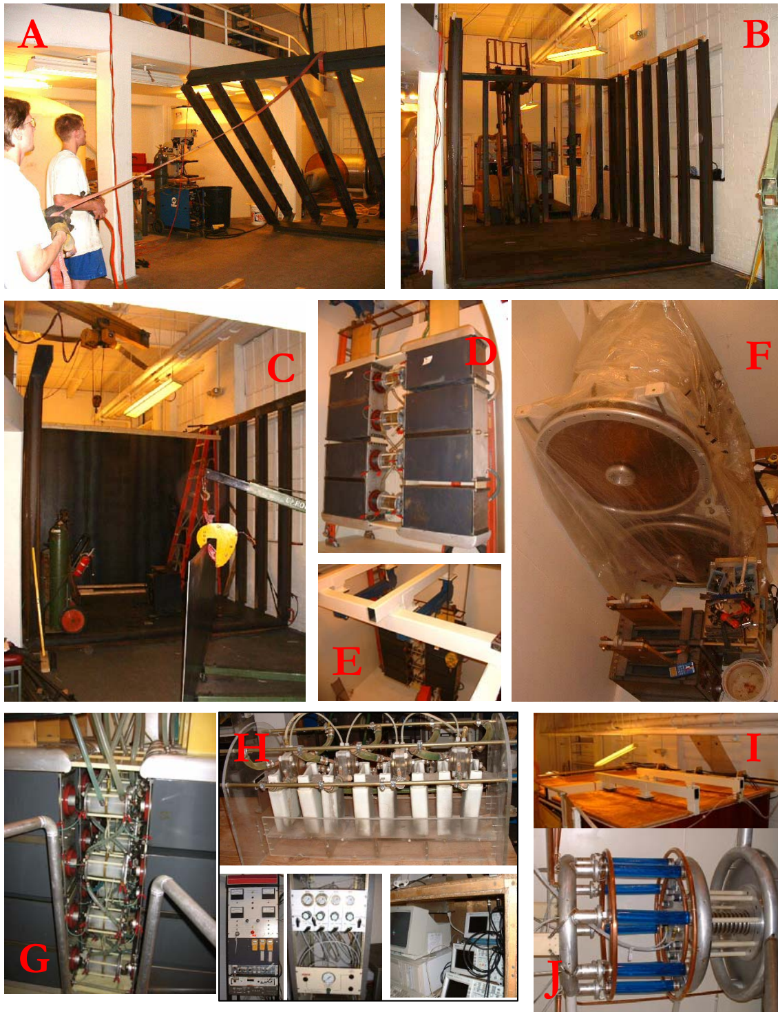
Fig. 9-3. Laboratory photographs. A) South wall assembly, B) Rib assembly, C) plate assembly, D) & E) Marx assembly, F) I-Store assembly, G) Marx complete, H) MTG assembly, control rack, gas rack, data acquisition system, I) Finished tank, J) Phase I output section.
