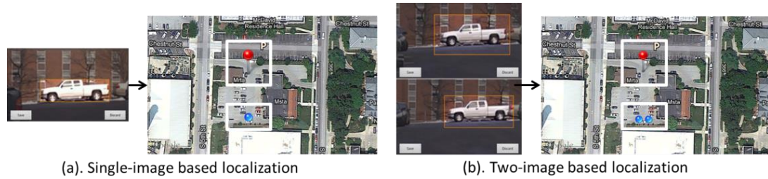
Figure 3.2. (a) Single-image based remote target localization: user takes a picture of a remote target and draws a tight bounding box around it; (b) Two-image based remote target localization: user inputs a rough bounding box on the left and right image enclosing the target. (The camera and the remote target positions are displayed on Google Maps. Blue dots: camera position; Red pin: estimated position of the remote target).
