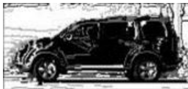
Figure 3.9. Black areas are Object patches with high confidence; White areas are Background patches with high confidence. Grey level areas are unclassified patches.
