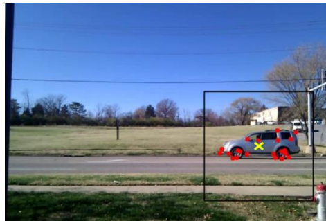
Figure 3.8. Yellow cross: user's tapping point; Black square: centered by user's tapping point with edge size D ; Red points: Lucas-Kanade optical flow features of the moving target.
