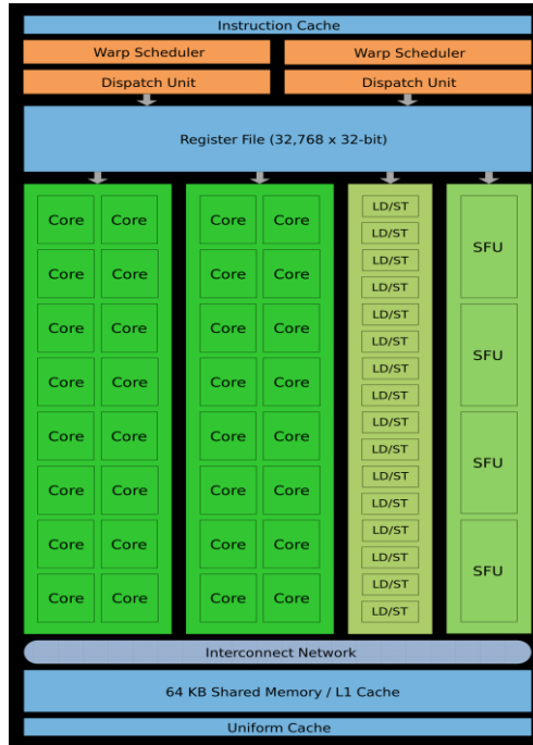
Fig. 2.3: Architecture of streaming multiprocessor on Fermi GPU.
