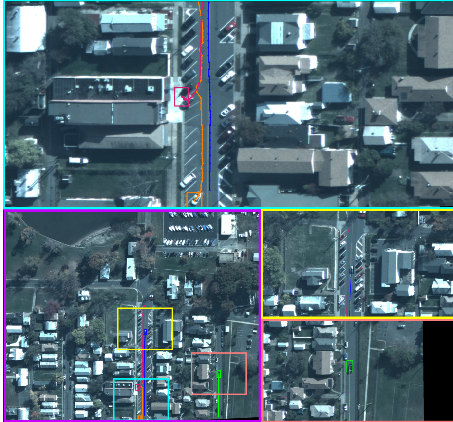
Figure 7.8: ARGUS-IS data showing LOFT tracks on frame #223 (full scene as in Left-Bottom (LB)-purple). Three zoomed up insets are marked with colored boxes (Right-Middle (RM)-yellow, Right-Bottom (RB)-light red, Top (T)-cyan) and each of them show the area that was zoomed into in the overview image (LB-purple). These tracking results were generated using LOFT-Hybrid ( min\_speed\_for\_da=3 ) configuration, same as Table 7.8. Notice that in the (T) inset the objects that are being tracked are those that were moving in the previous time steps and are now stationary while two other moving objects (RM) & (RB) are in motion showing the adaptive integration of appearance and motion model. This illustration was shown in Bashrat et al. [88]
