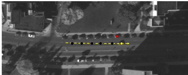
Figure 3.4: When the maximum peak (red dot) deviates from the smooth trajectory assumption (in this case linearity) LOFT ignores the distractor to select a less dominant peak satisfying the linearity constraint (yellow dot) [42].
