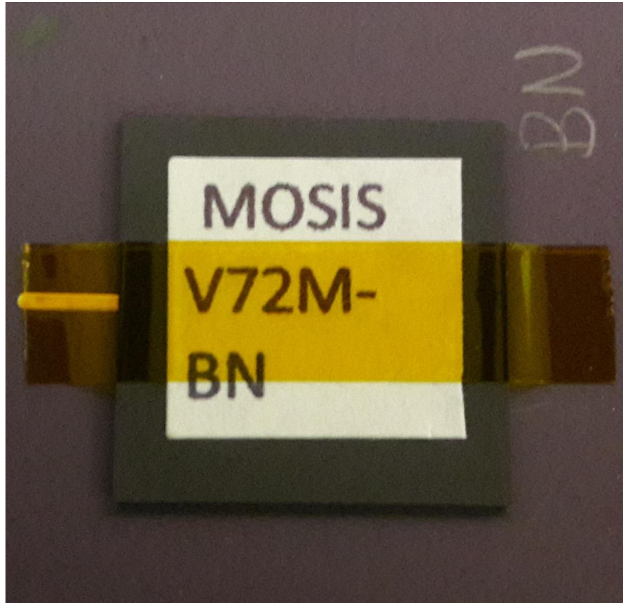
Figure 8.2: Picture of the fabricated chip containing HLDR, SVR, and all three PMS designs
