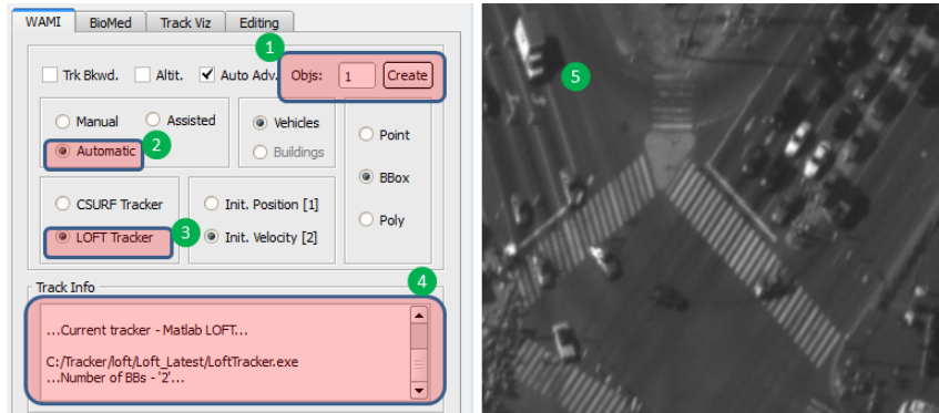
Figure 8.10: Step I of tracking an object using the LOFT Tracker. The user first creates a new Object-ID (Highlighted by rounded rectangle 1). Creating a new Object-ID in KOLAM always sets the Tracking Mode to Automatic (2) and sets CSURF as the selected tracker. The user needs to change the tracker to LOFT (3). KOLAM gives the user feedback and the next step to perform in the tracking process (4). The object (vehicle in this case) to be tracked is also highlighted (5).
