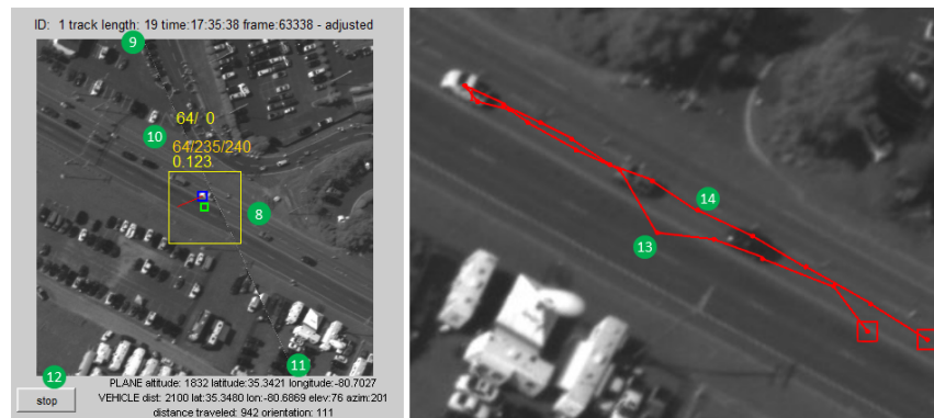
Figure 8.9: Step III of tracking an object using the CSURF Tracker. Once initialized, the CSURF program begins tracking the object (8). While tracking, CSURF presents additional useful information to the user (9, 10, 11) as well as the means to terminate itself (12). The trajectories for the object - unregistered (13) and registered (14) - are drawn in KOLAM as soon as they are generated by the tracker.
