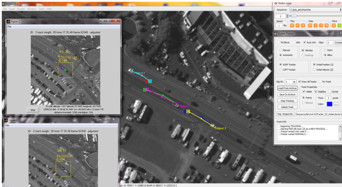
Figure 3.12: Simultaneous visualization of tracker algorithm execution and trajectory visualization in KOLAM. There are three instances of the tracking algorithm running to track three objects. The two inlaid (MATLAB) windows shown on the left are the realtime (heads-up or cursor-on-target) displays generated by the automatic tracking algorithms. The main window shows both stabilized and unstabilized computed trajectories for the three objects.
